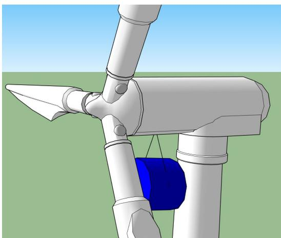
Figure 3.15: Supported pulley hoist
