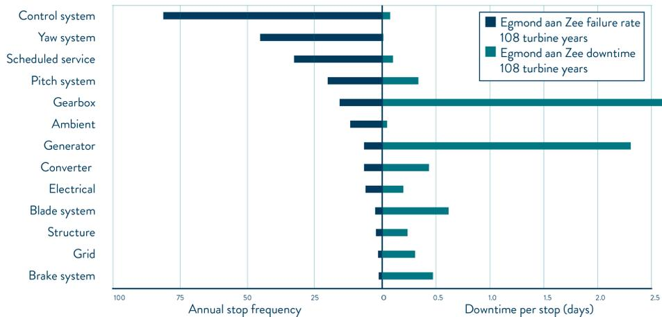
Figure 2.5: Offshore reliability of OWEZ wind farm<sup>[5]</sup>
