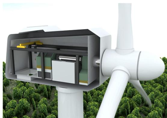
Figure 3.12: Integrated overhead crane
