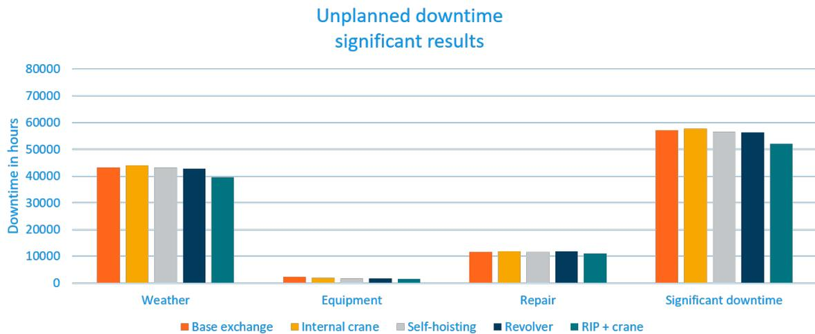
Figure E.4: Significant downtime per mechanism for 5.0 MW “Hollandse Kust: Noord-Holland”
