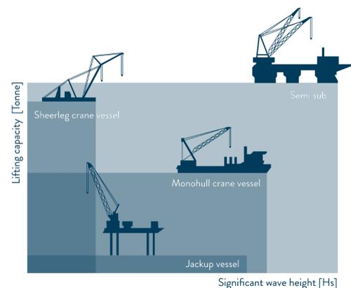
Figure 2.10: Service vessel operationality
