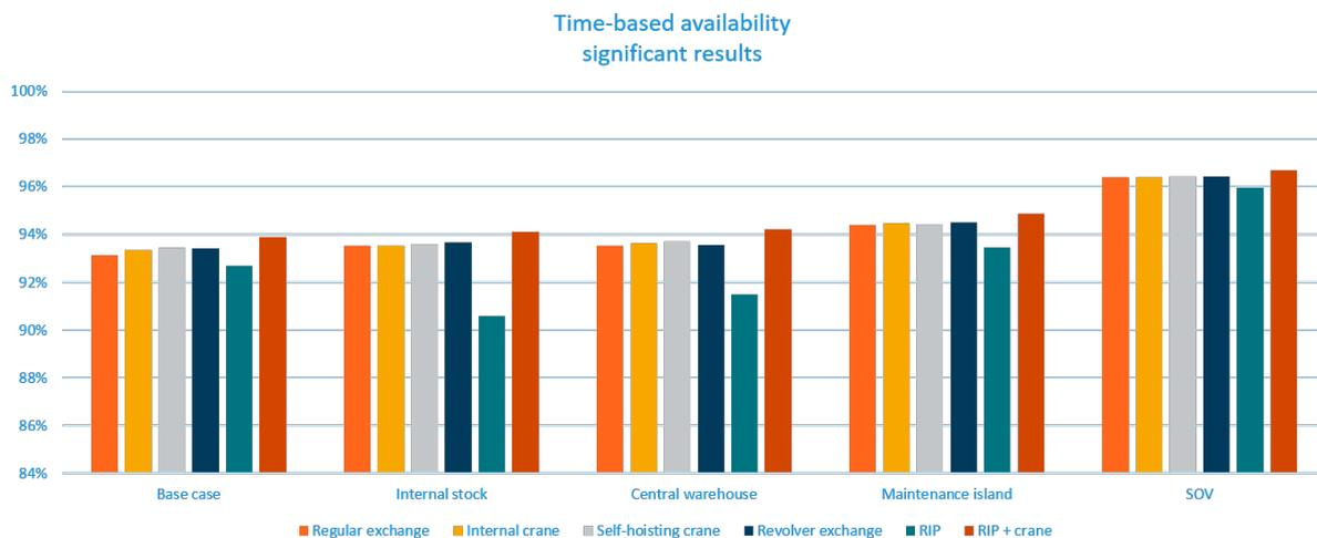
Figure 5.8: Significant time-based availability per exchange mechanism
