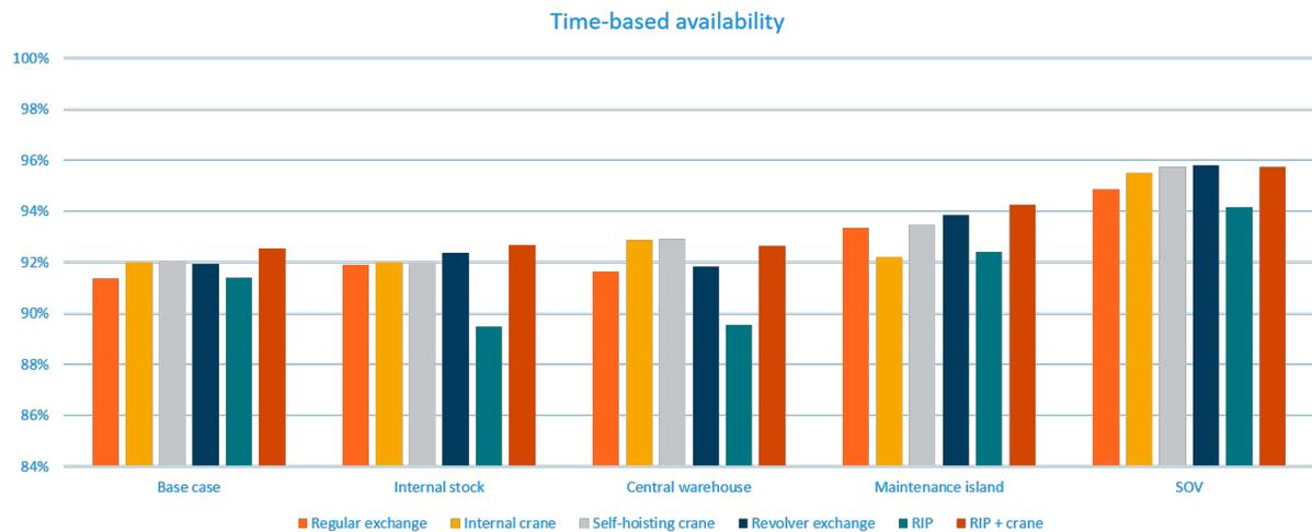
Figure 5.6: Time-based availability per exchange mechanism
