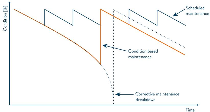
Figure 2.3: CBM compared to FBM and TBM<sup>[3]</sup>
