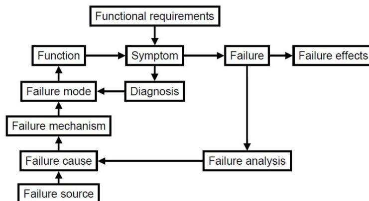
Figure 2.1: Terminology of failures<sup>[1]</sup>
