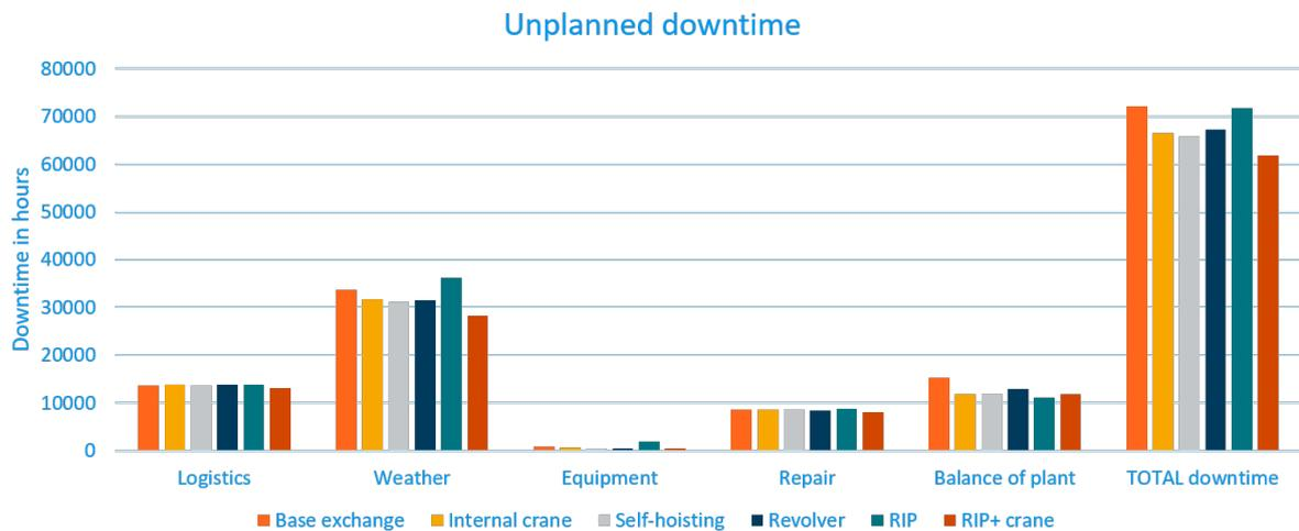
Figure 5.3: Downtime specification per exchange mechanism
