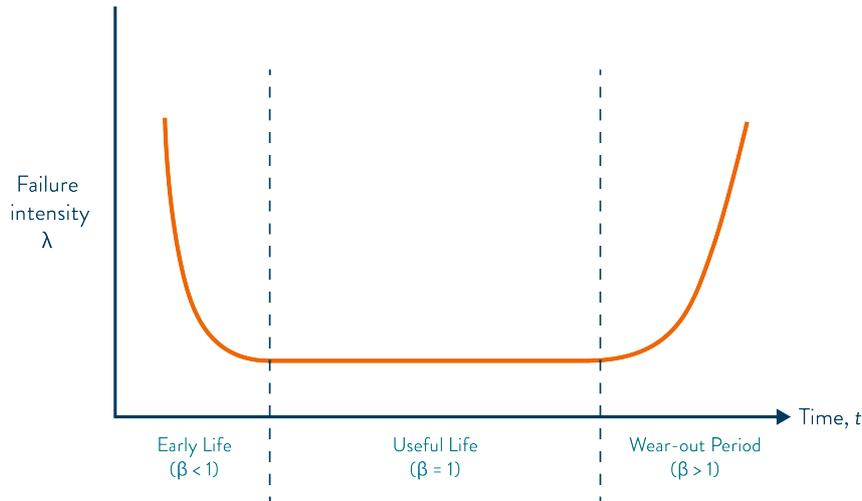
Figure 2.8: Bathtub curve for mechanical components<sup>[4]</sup>
