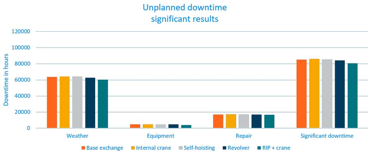
Figure E.6: Significant downtime per mechanism for 5.0 MW “IJmuiden Ver”
