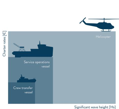
Figure 2.9: O&M vessel operationality
