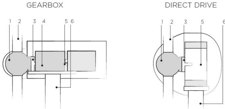
Figure 1.1: Conventional wind turbine configurations
