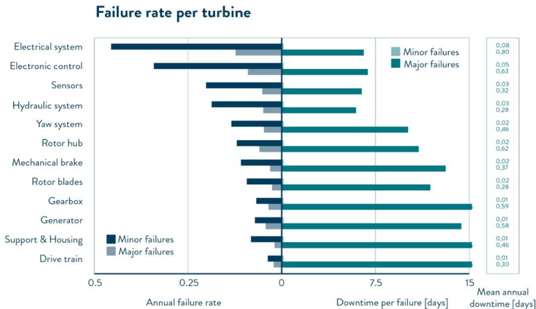
Figure 2.7: MTTF-MTTR according to failure<sup>[7]</sup>
