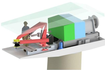
Figure 3.11: Knuckle boom crane
