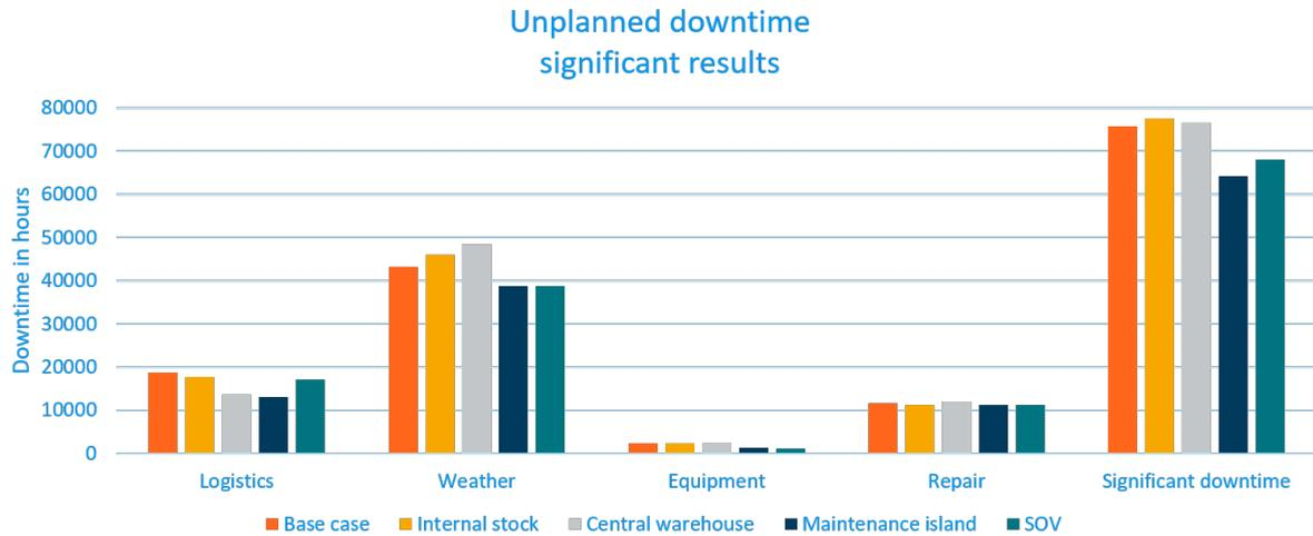
Figure E.3: Significant downtime per scenario for 5.0 MW “Hollandse Kust: Noord-Holland”
