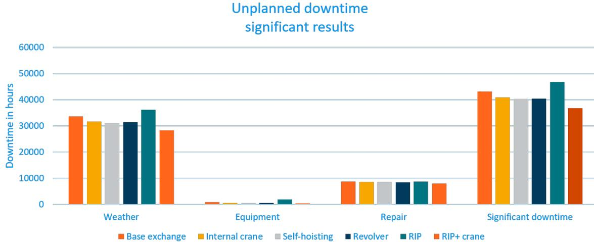
Figure 5.4: Significant downtime specification per exchange mechanism
