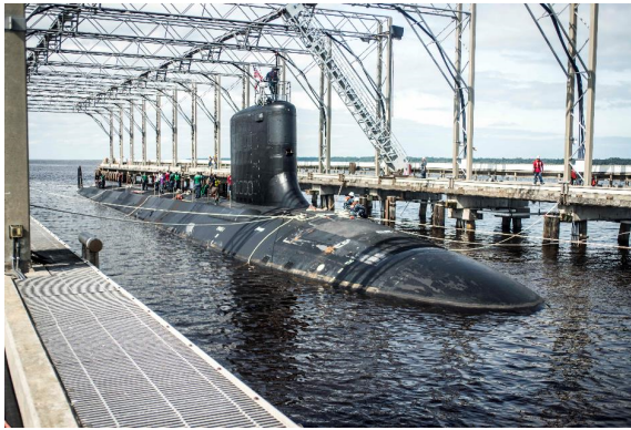
(a) The USS West Virginia undergoing a deperming treatment in the drive-in facility of the Naval Submarine Base Kings Bay. Source: United States Navy
