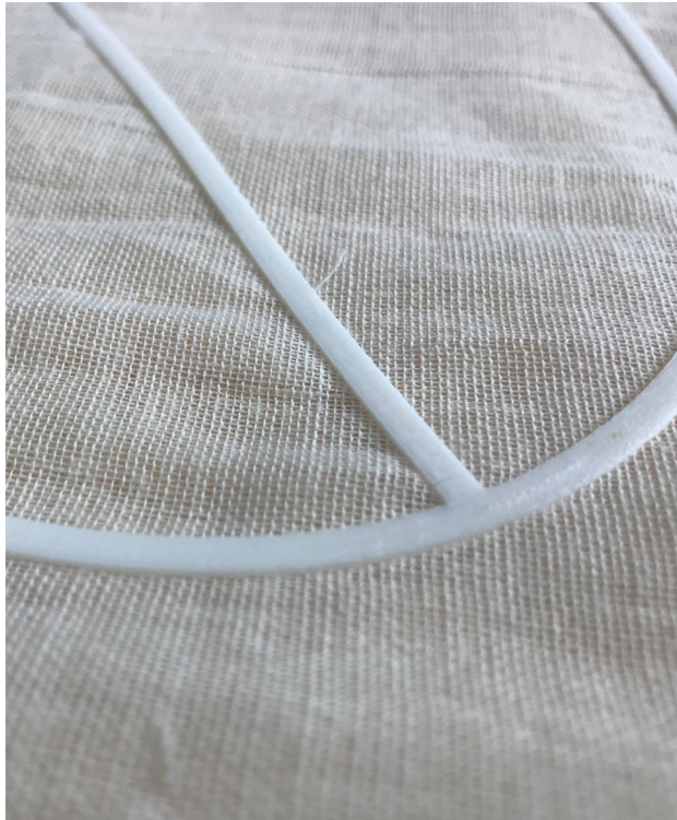
Figure 94 Close up of UM TPU 95A printed on mesh cotton
