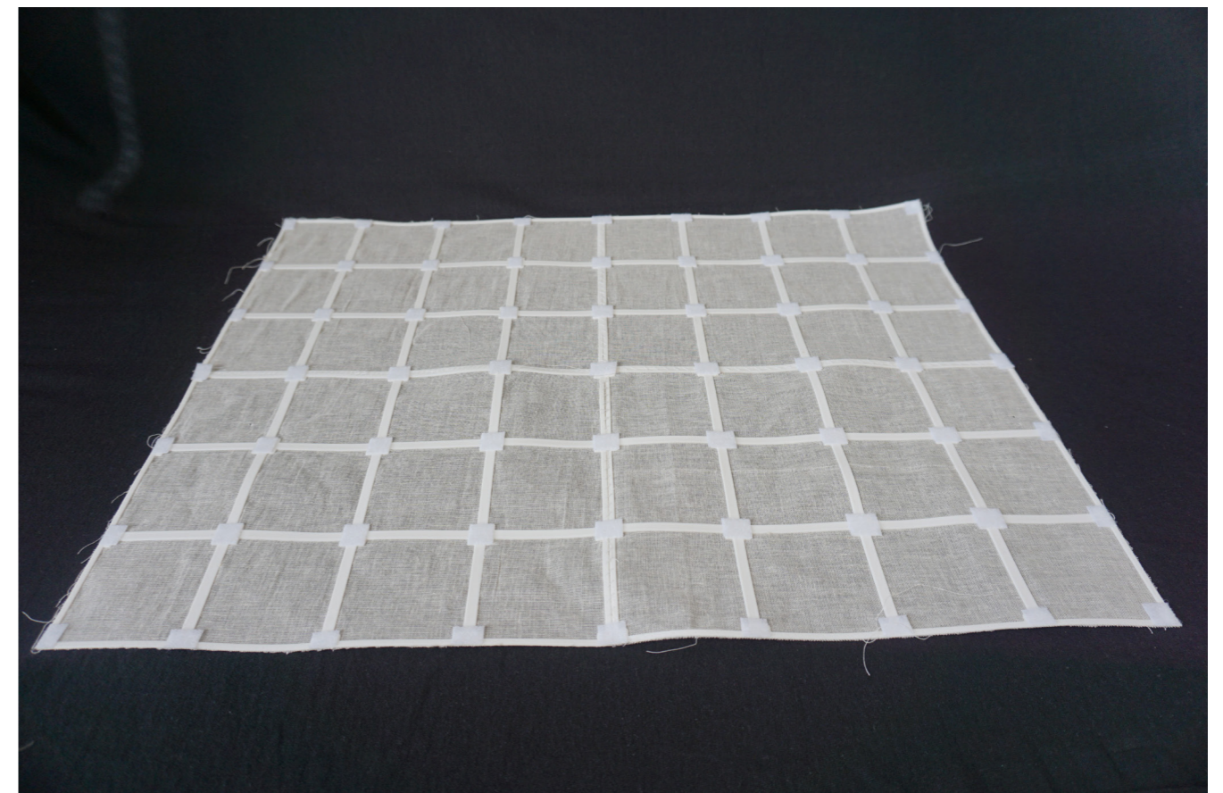
Figure 123 Connecting modular toolkit modules together with sewing method
