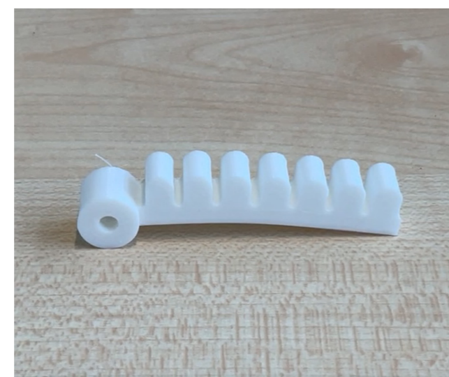
Figure 50 Improved actuator with new printer settings
