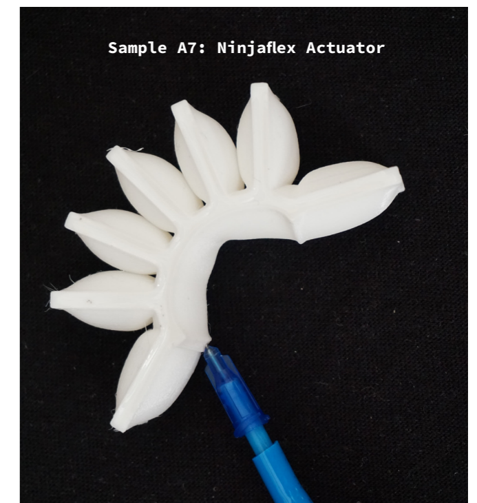
Figure 73 Prototype replicating morpheesPlug settings
