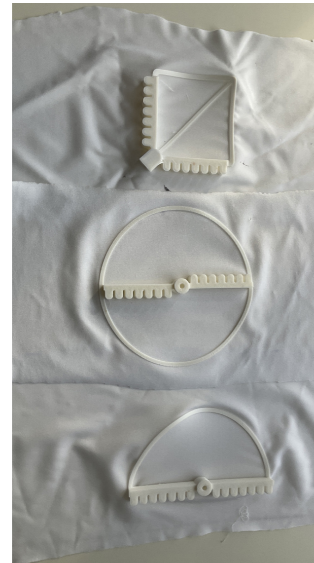
Figure 51 Actuators printed on textile prototypes
