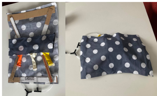
Figure 43 Textile sheet actuator with skeleton structure prototype
