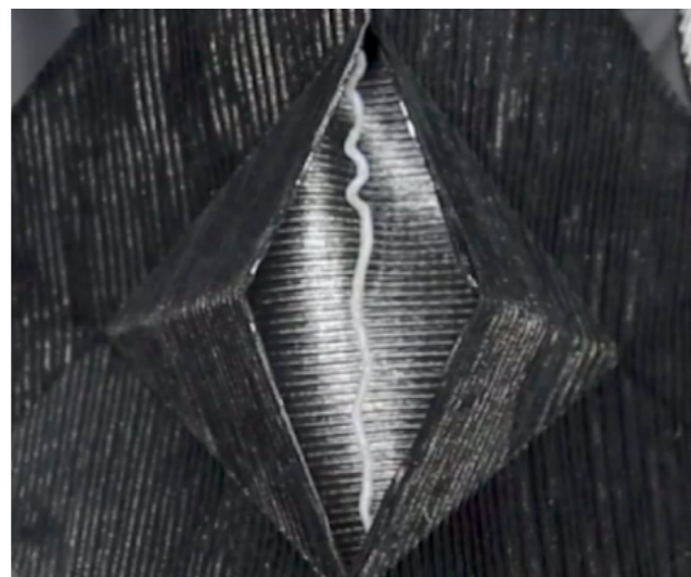
Figure 20 ModiFiber: a reversible SMA actuator (Forman et al., 2019)
