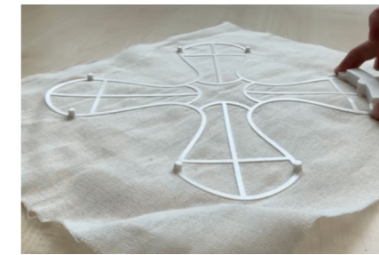
SAMPLE T15: Jellyfish Dome Material: UM TPU 95A Print height: 1,5mm Print width: 2,5mm
