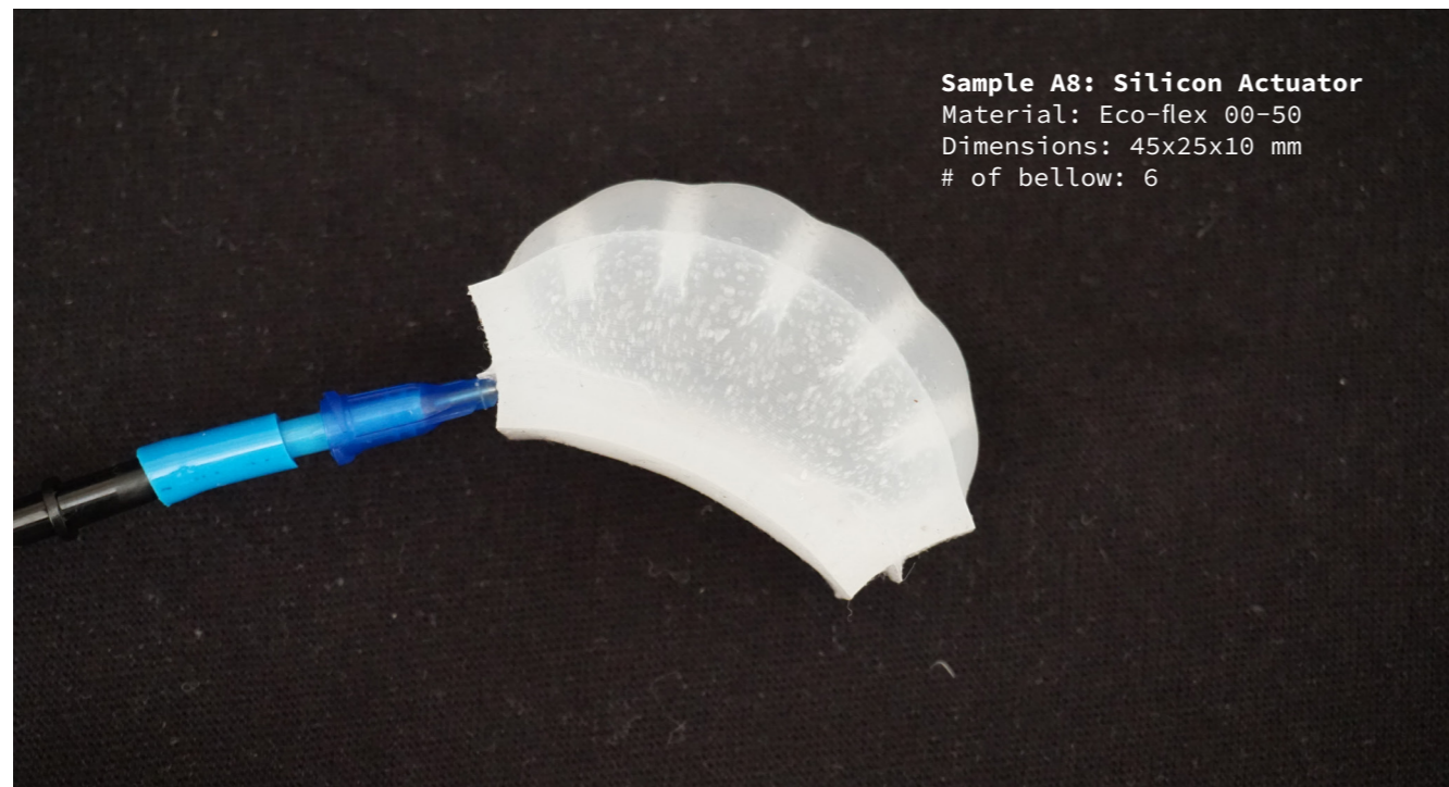
Figure 75 Silicon casted actuator (Eco-flex 00-50)
