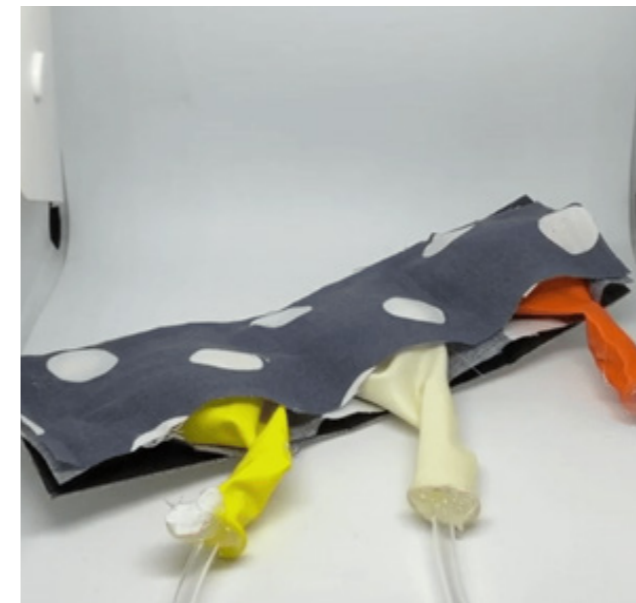
Figure 41 Bending actuator built with balloons and textile
