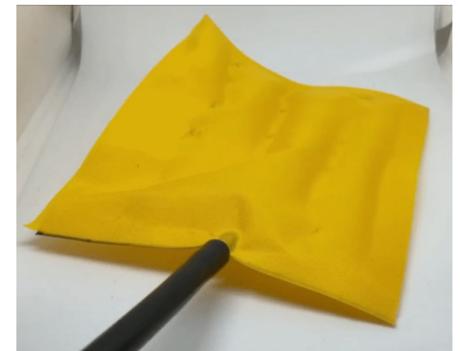
Figure 44 Heat sealed textile inflatable prototypes
