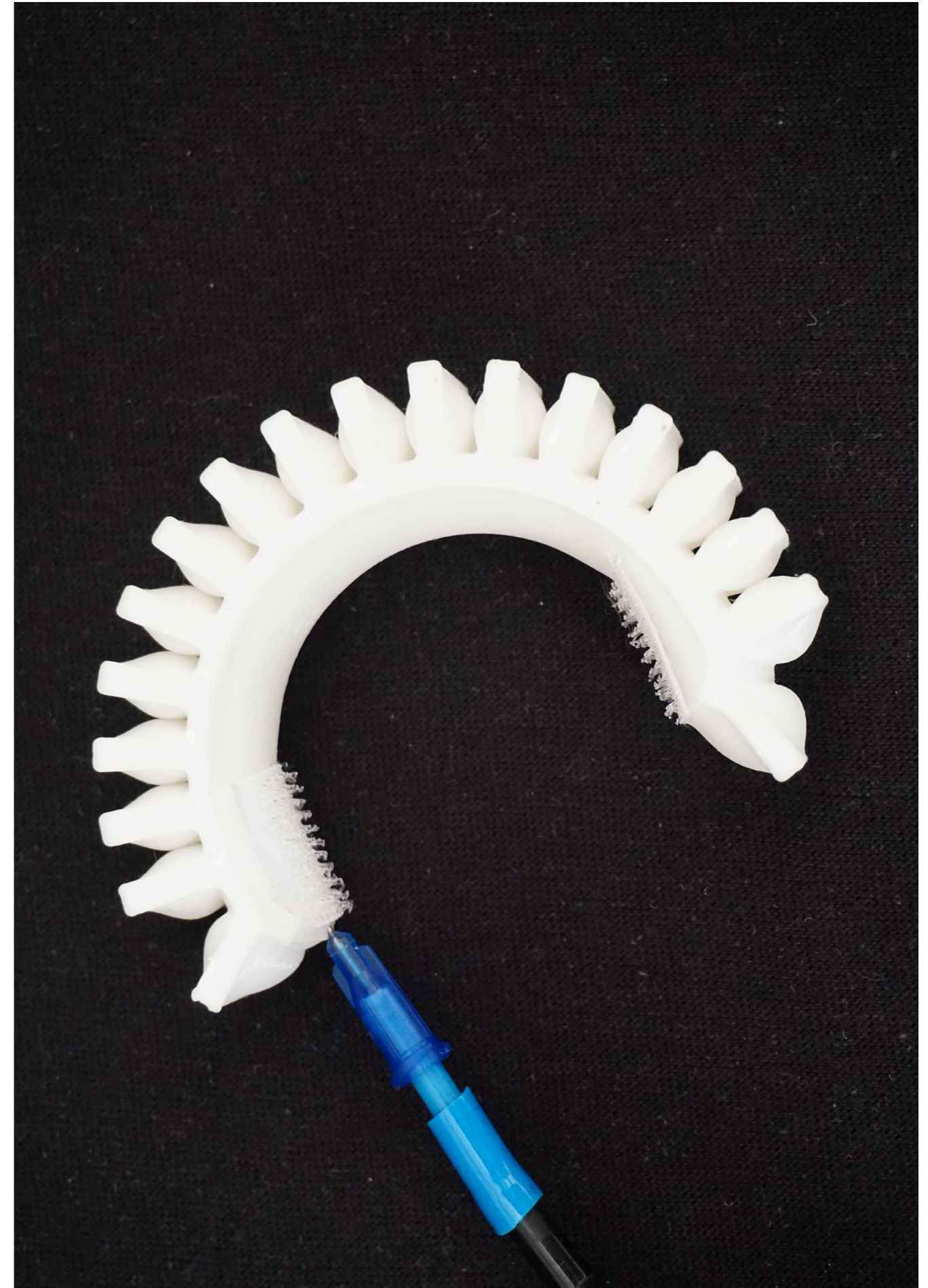
Figure 98 Sample A13 actuator in its actuated state
