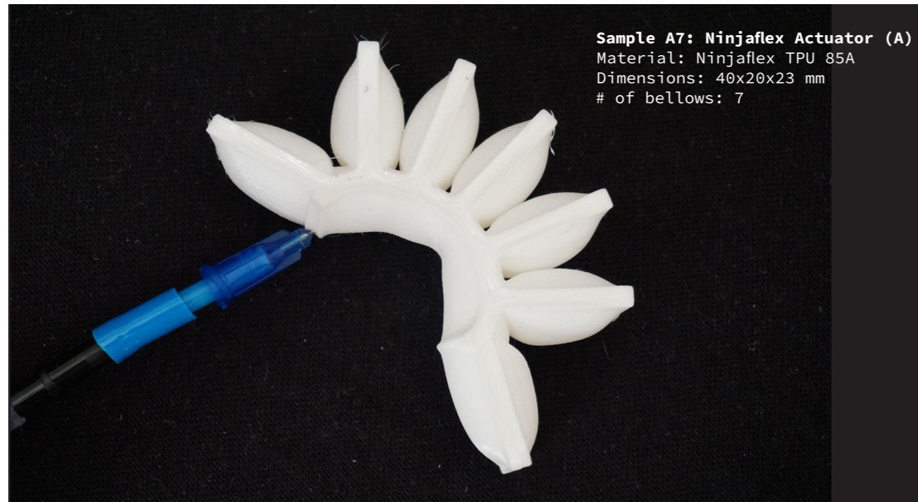
Figure 74 3D printed actuator (Ninjaflex TPU 85A)
