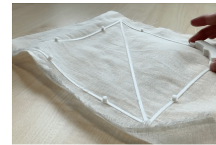
SAMPLE T14: Wings Material: UM TPU 95A Print height: 1,5mm Print width: 2,5mm
