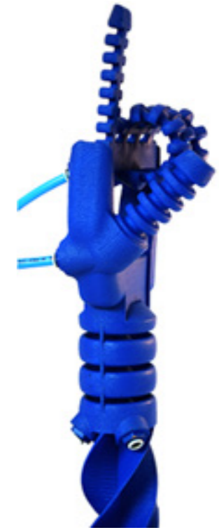
Figure 48 Pneumatic soft robotic hand (Scharff et al., 2017)
