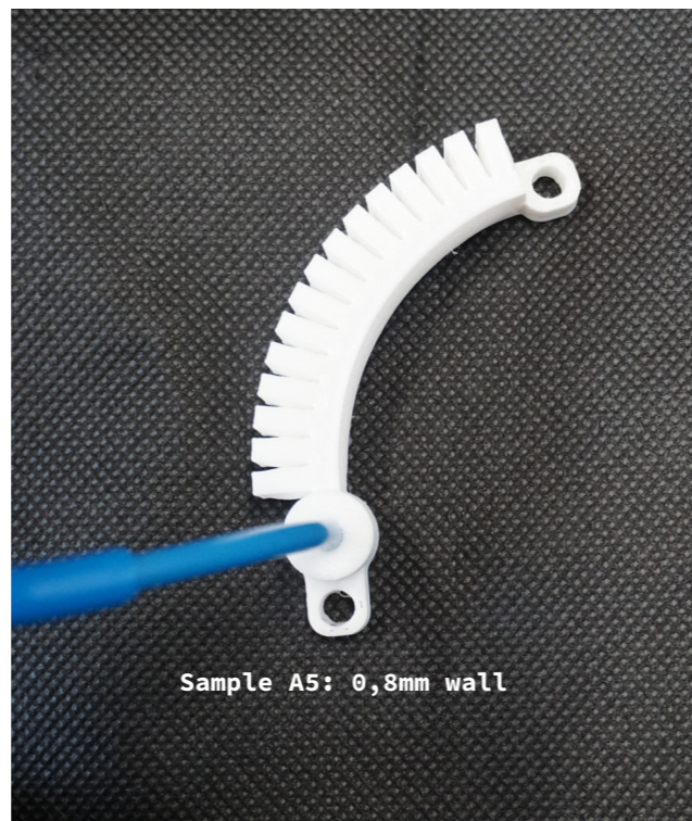
Figure 67 Actuator with 0,8mm wall thickness actuated
