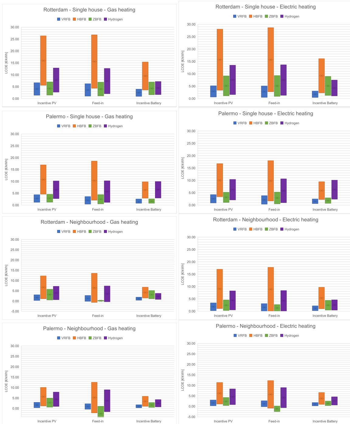
Figure 5.7: LCOE results collection in different future incentive scenarios for each battery type
