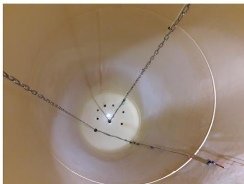
Figure 6.2: The wire thermocouple used in Haakh’s experiment measurements (Haakh, 2022)
