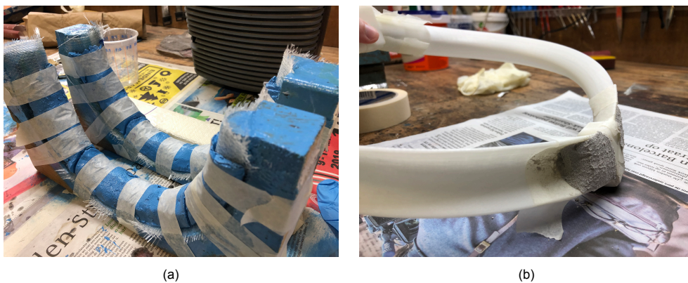
Figure 3.2: (a) GFRP clamped between an inside and outside mold, (b) shaping the inside mold from the 3D print
