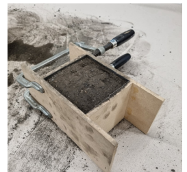
Fig. 39 Rammed earth making process photograph (own image, 2022)
