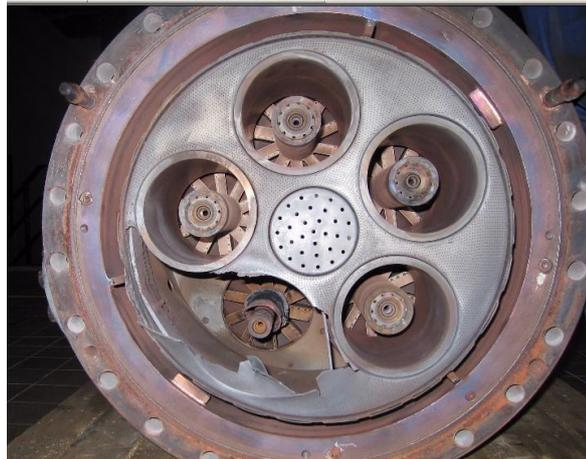
Figure 1.6: Damaged cover on a gas turbine burner due to excessive combustion dynamics [24]
