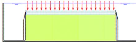
Figure A.27: Terzaghi's problem representing an oedometer test, after Verruijt (2013)
