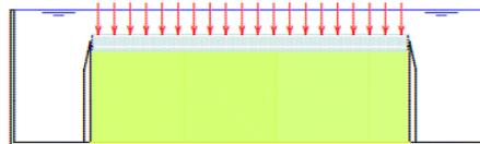
Figure 2.6: Terzaghi's problem representing an oedometer test, after Verruijt (2013)
