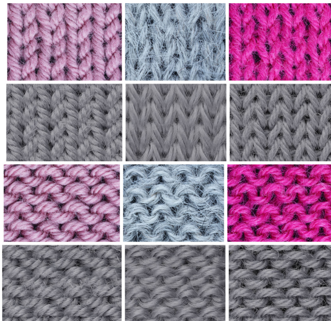
Fig. 9. 1st and 3rd rows: images of a real knitted cloth (made with yarns from the top row of Fig. 10) for the pattern consisting of knit (1st row) and purl (3rd row) stitches. 2nd and 4th rows: rendering of the same stitch pattern with the inferred yarn with default material settings.
