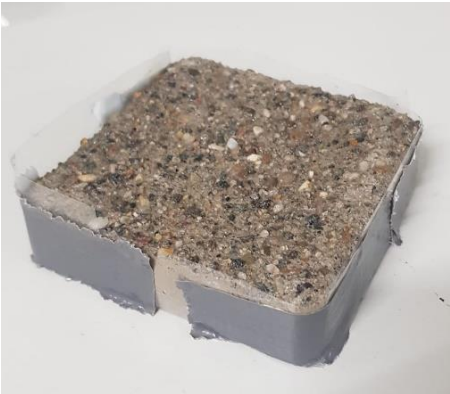
Figure 4.6: Concrete sample wrapped in plastic foil
