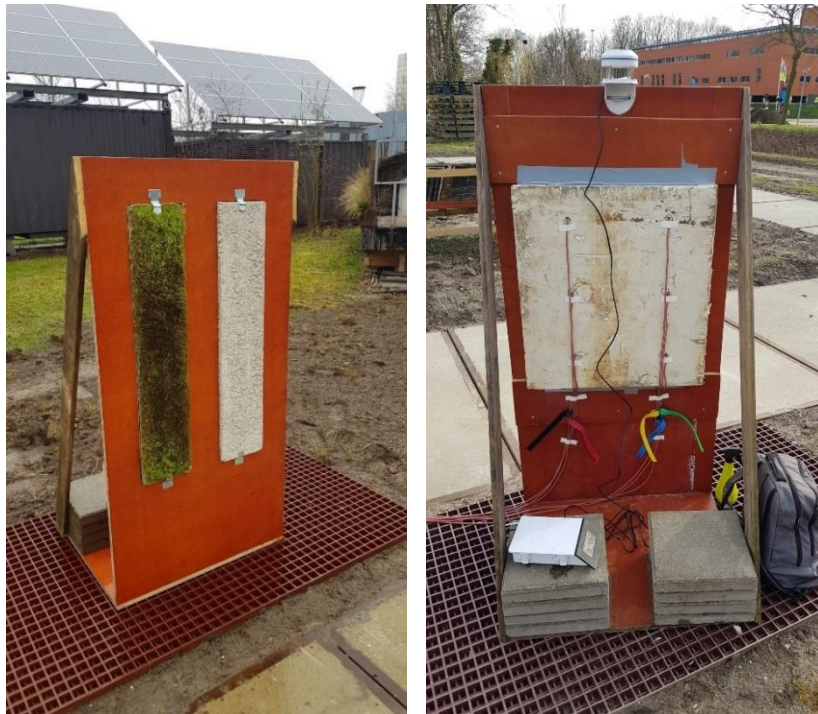
Figure 5.1: Front and back view of the frame with mounted façade panels and measuring equipment
