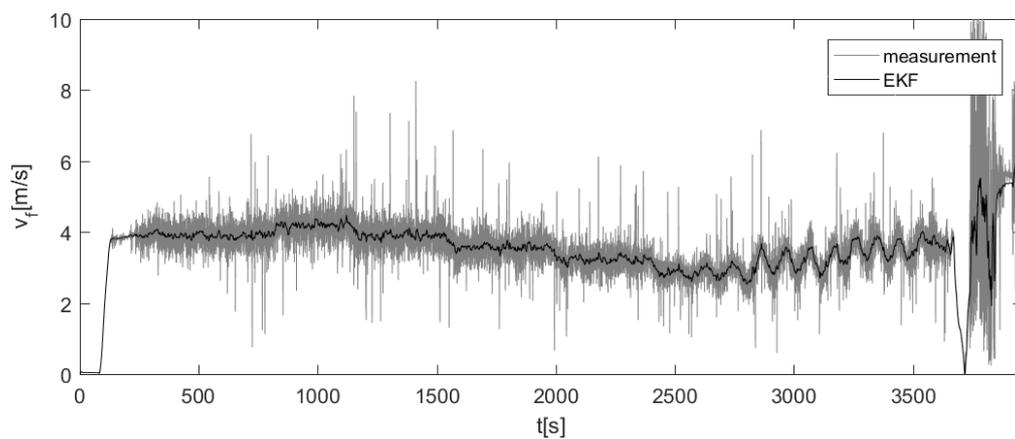
**Figure C-10:** Estimated fluid velocity ( $v_f [m/s]$ ), measurement 10
