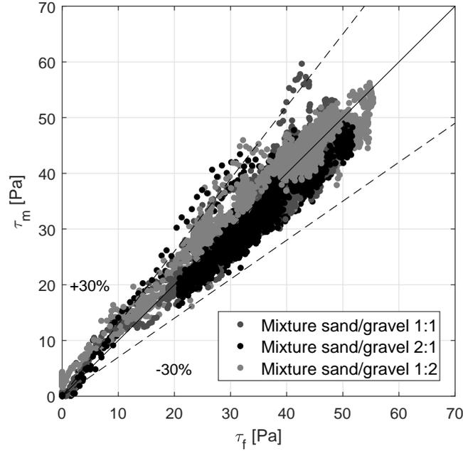
**Figure 4-16:** Validation of mixture shear stress
