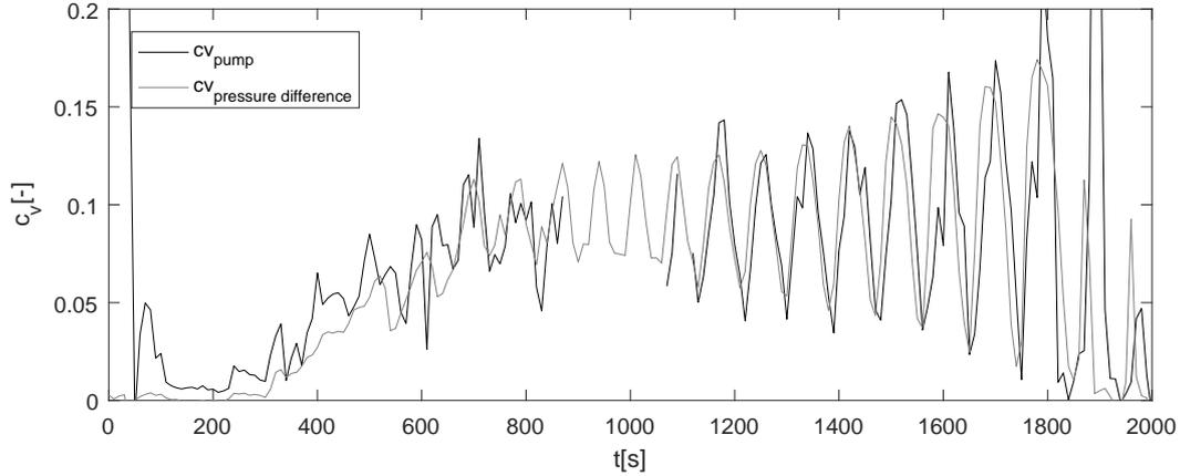
**Figure 4-3:** Measured concentration using pump efficiency decrease, and  $\Delta p$  measurement.
