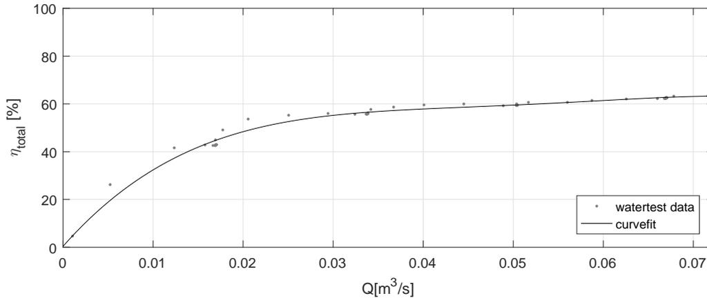
**Figure 4-2:** Total efficiency: measured data and curvefit
