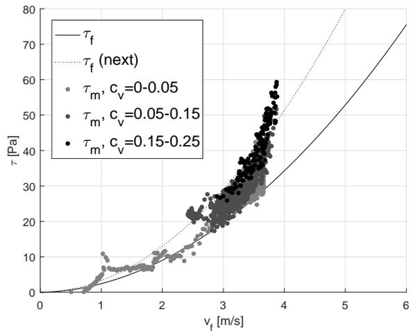
**Figure 4-13:** Measured wall shear stress, measurement 5 (gravel,  $c_v = 0.15$ )
