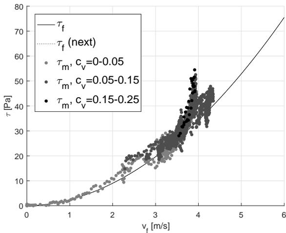
**Figure 4-12:** Measured wall shear stress, measurement 4 (gravel,  $c_v = 0.10$ )
