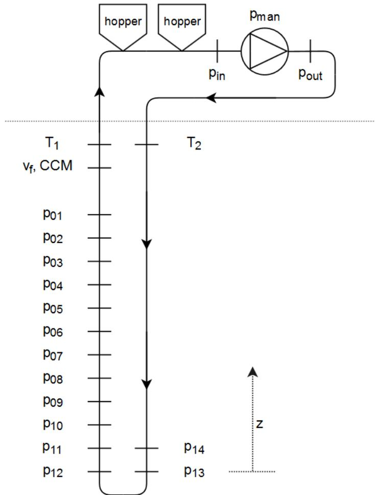
**Figure 3-5:** Schematic representation of the test setup
