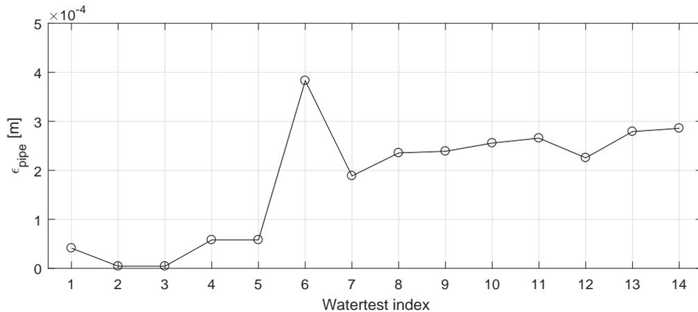
**Figure 4-5:** Pipe wall roughness found for different watertests
