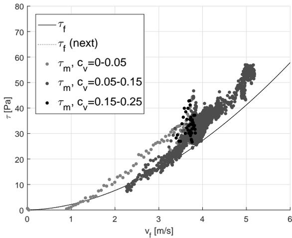
**Figure 4-8:** Measured wall shear stress, measurement 2 (sand,  $c_v = 0.05$ )
