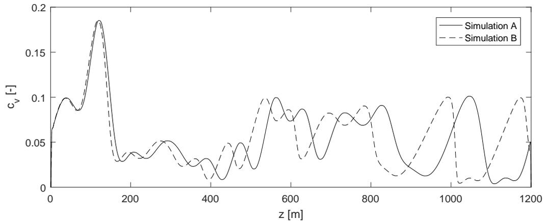
**Figure 2-6:** Simulated concentration in riser at  $t = 500s$ , case A and B
