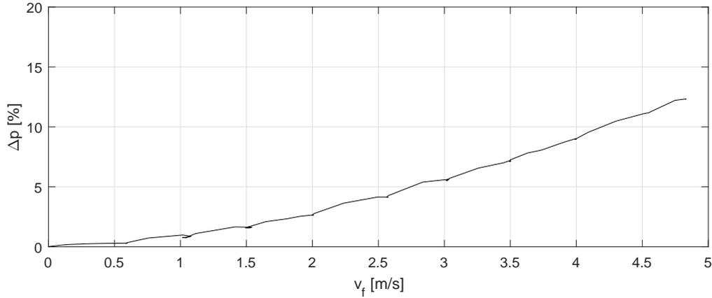
**Figure 4-4:** Relative pressure drop due to wall friction
