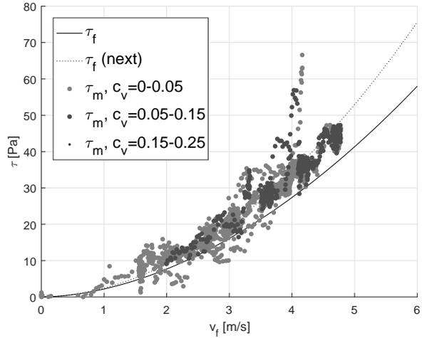
**Figure 4-11:** Measured wall shear stress, measurement 3 (gravel,  $c_v = 0.05$ )
