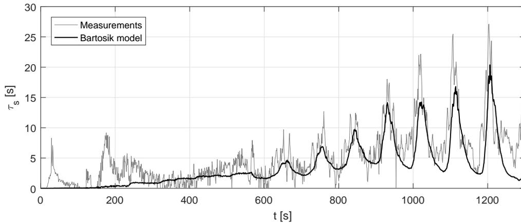
**Figure 4-14:** Validation of measured mixture shear stress with the model proposed by Bartosik
