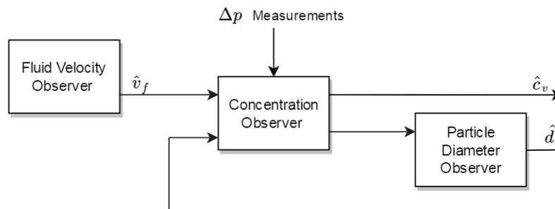
**Figure 1-4:** Simplified Observer Structure
