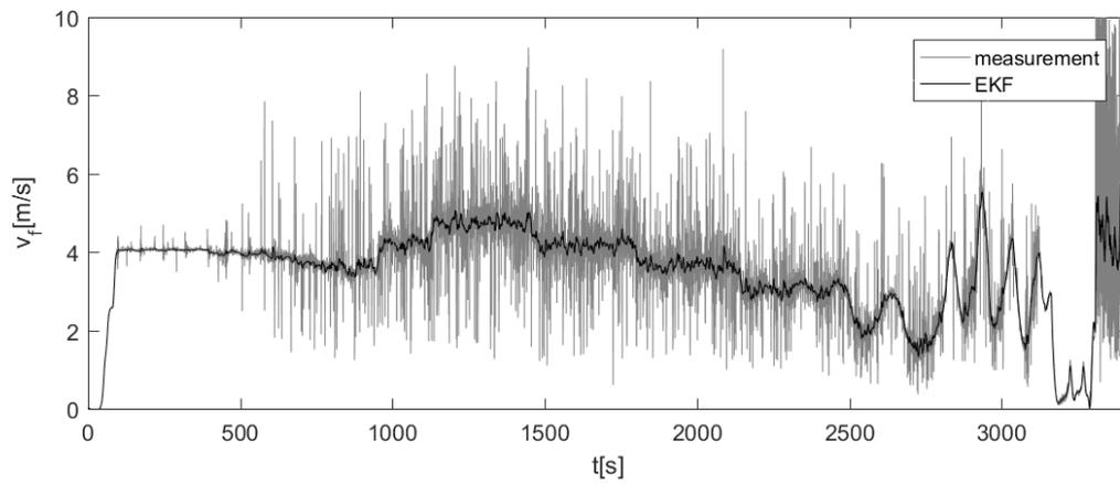
Figure C-3: Estimated fluid velocity ( $v_f [m/s]$ ), measurement 3
