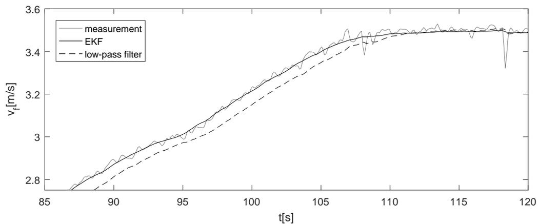
**Figure 5-4:** Comparison of EKF and low-pass filter applied on measurement 4
