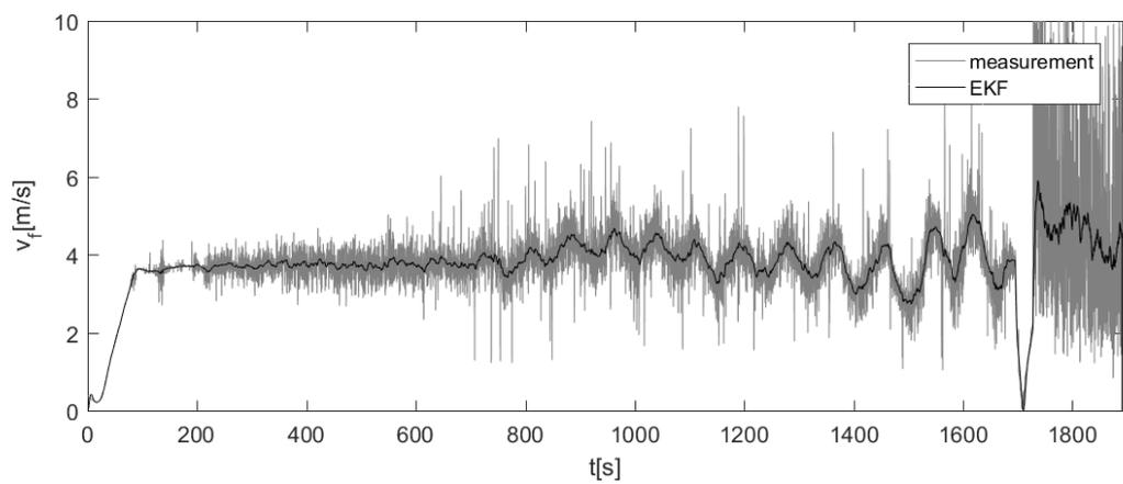
**Figure C-7:** Estimated fluid velocity ( $v_f [m/s]$ ), measurement 7
