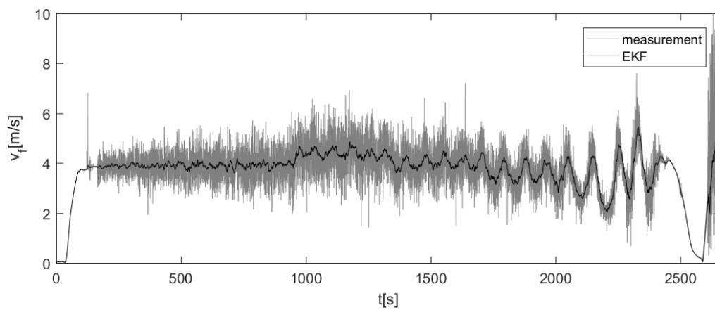
**Figure C-13:** Estimated fluid velocity ( $v_f [m/s]$ ), measurement 13
