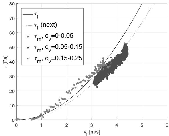
**Figure 4-9:** Measured wall shear stress, measurement 6 (sand,  $c_v = 0.10$ )
