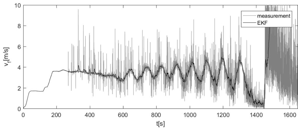
**Figure C-5:** Estimated fluid velocity ( $v_f [m/s]$ ), measurement 5
