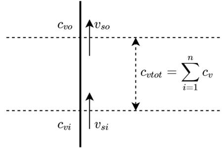
**Figure 5-12:** Selected riser section with ingoing and outgoing flux.
