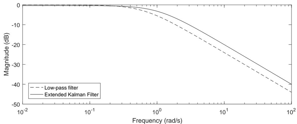
**Figure 5-6:** Magnitude plot of of EKF and low-pass filter
