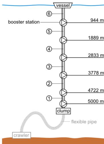
**Figure 1-2:** Vertical Transport System (VTS)
