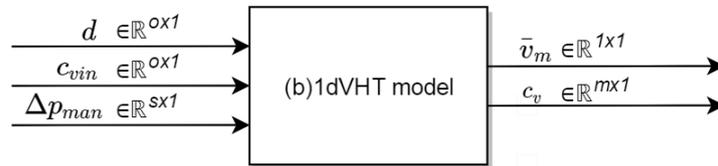
Figure 2-1: Input-output scheme of the (b)1DVHT model
