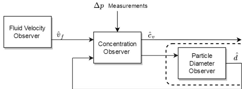
**Figure 5-10:** Simplified Observer Structure
