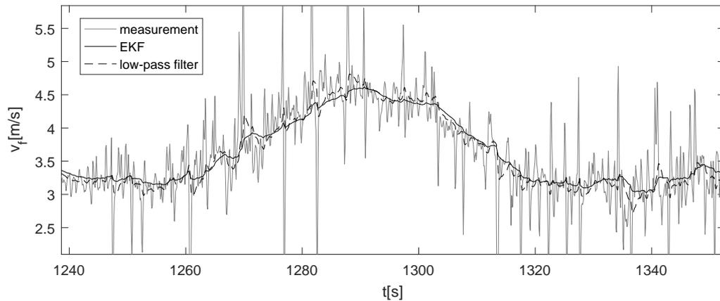
**Figure 5-5:** comparison of EKF and low-pass filter applied on measurement 4
