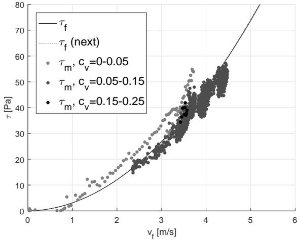
**Figure 4-10:** Measured wall shear stress, measurement 13 (sand,  $c_v = 0.15$ )
