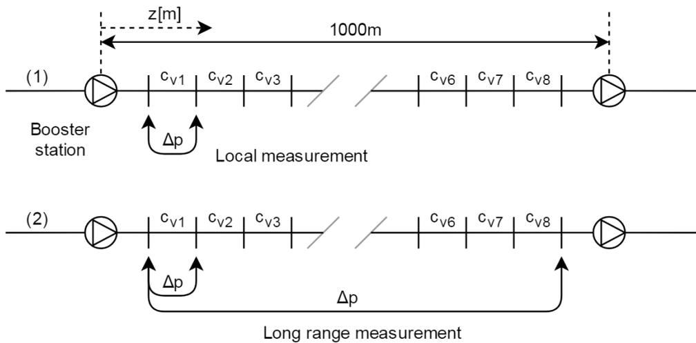
**Figure 2-2:** Measurement configuration 1 and 2
