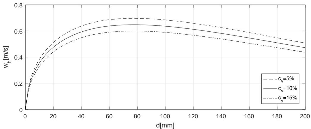
Figure 5-11: Hindered settling velocity.
