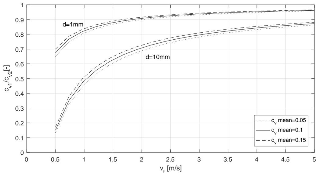
**Figure 4-7:** Ratio between the concentration in a riser and the downcomer, for different particle diameters
