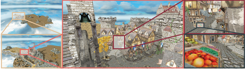
Figure 2.1: Compressed voxelized scene at different levels of detail, rendered in real time using raytracing only. Our hierarchy encodes geometry and quantized colors at a resolution of 128K^3 . Despite containing 18.4 billion colored nodes, it is stored entirely on the GPU, requiring 7.63 GB of memory using our compression schemes. Only at the scale shown in the right bottom image the voxels become apparent.
