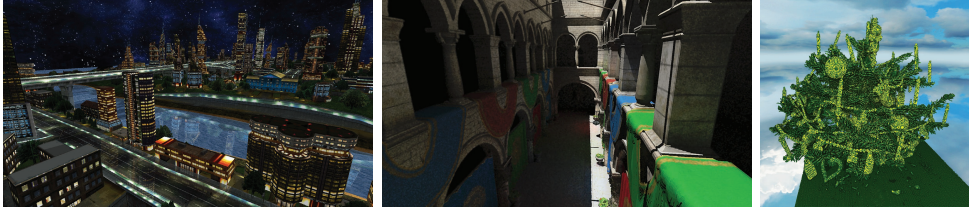
Figure 2.8: Several applications of our compressed SVO. From left to right: encoding reflectance information in materials for the City scene, rendered at a resolution of 32K^3 ; color bleeding in the Sponza scene, at an SVO resolution of 4K^3 , using 16 samples per pixel, and secondary and tertiary ray tracing at a 512^3 resolution; rendering of the dense Christmas Tree dataset at a 512 \times 512 \times 999 resolution.
