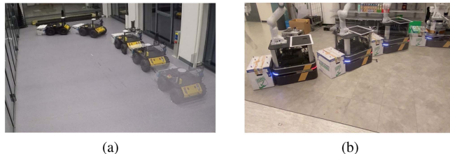
Fig. 1. Wheeled mobile robots (Clearpath Husky and Boxer) push a letter box to a goal location and to track a reference path, respectively. Transparency of the robots and box indicates their movement.
