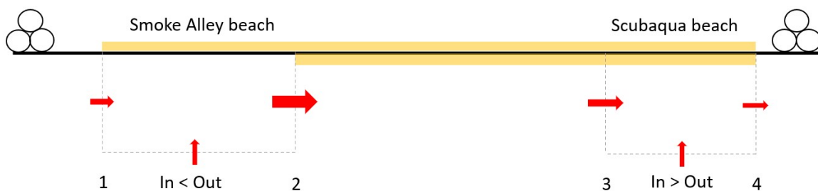
Figure 4.5: Sediment budget after storm Earl for Smoke Alley beach and Scubaqua beach related to Figure 4.4c
