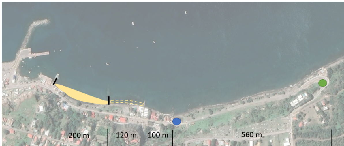
Figure 5.6: Illustrative sketch of Alternative I. The nourishment is coloured in yellow and the possible extension is noted with a dashed line. The location of Scubaqua is highlighted with a blue circle and the location of Smoke Alley with a green circle.
