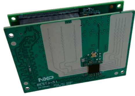
Fig. 1. A credit card size automotive radar system that is used for experiments: NXP TEF810X / S32R274 Radar Chipset
