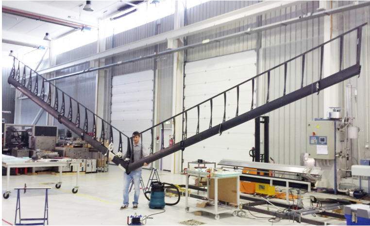
Figure A.11 | Prototype rigid wing skeleton pictured during assembly [80, 191].
