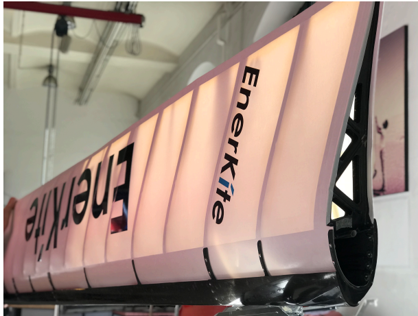
Figure A.12 | Prototype fixed-wing kite structure with carbon skeleton and textile covering (image courtesy EnerKite).
