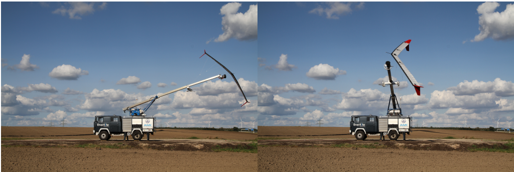
Figure A.7 | EnerKite technical demonstrator system comprising a mobile base station with a rotational landing and launching mast, pictured during a launching operation with a prototype wing [80].
