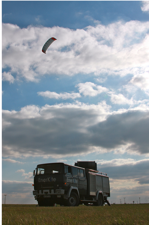
Figure A.2 | The EK30 mobile technology demonstrator in operation with the early generation soft-wing kites (circa 2013, image courtesy of EnerKite).
