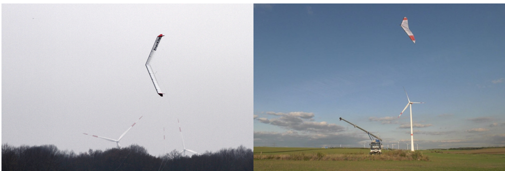
Figure 1.9 | Swept fixed wing prototype(s) in flight with the EK30 technical demonstrator (circa 2015-2022, images courtesy of EnerKite).
