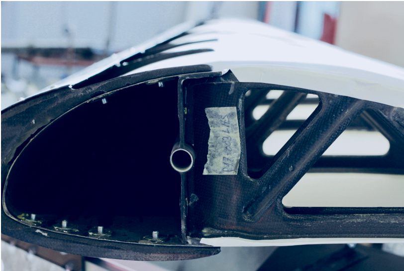
Figure 4.4 | Early prototype wing box formed by atypical D-box positioned at the leading edge (circa 2016, image courtesy of EnerKite).
