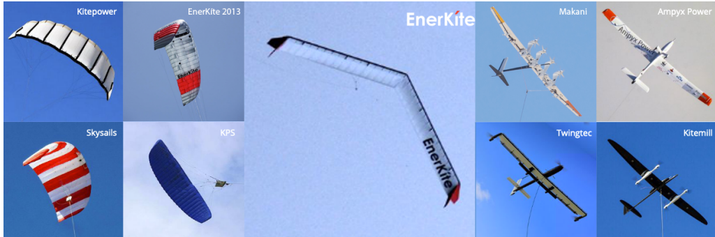
Figure 2.1 | Various commercial AWE systems with kite-like and aircraft-like airborne systems. Adapted from [33].
