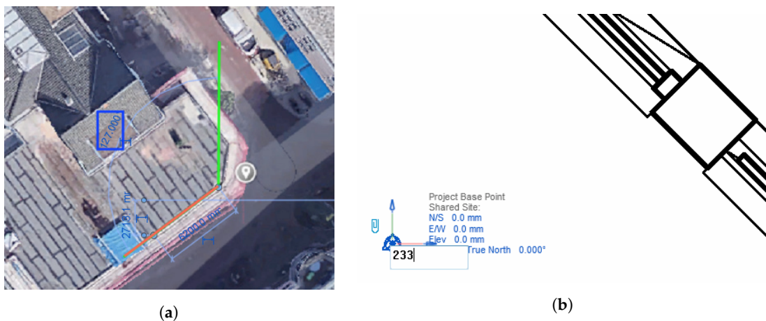
Figure 18. Detection and correction of an IFC file's TrueNorth . (a) Finding of the angle between the true north (green line) and the project north (orange). (b) Correction of the Project Base Point's True North attribute.
