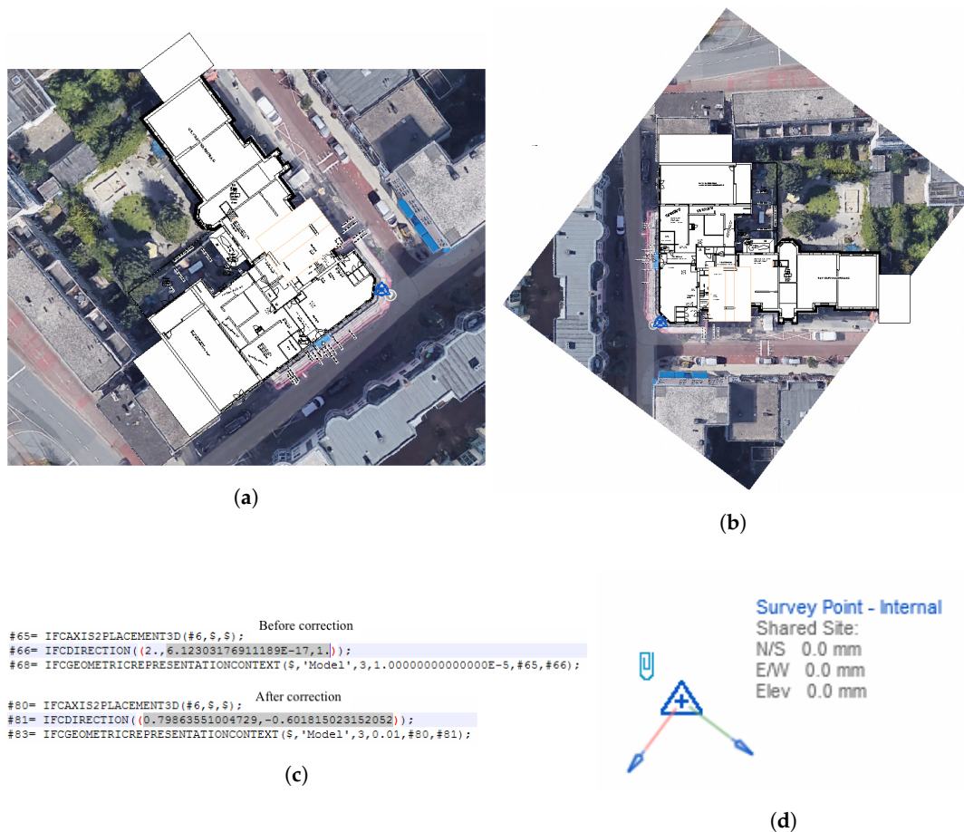
Figure 19. (a) Superposed floor plan and image oriented with respect to the true North; (b) Superposed floor plan and image oriented with respect to the project North; (c) New IfcDirection of the true north; (d) New Survey Point of the project.
