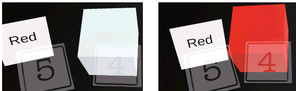
(a) A variable marker containing a cube object before moving close to the red action marker. (b) The variable marker after moving close to the red action marker. The colour of the cube was changed to red.
