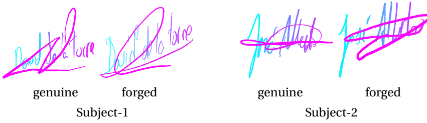
Figure 1.2: Signature examples from MCYT_Signature corpus [1]. We visualize two groups of signatures from two subjects, each group includes one genuine and one forged signature. For each signature, the pen moves from cyan color to magenta color. Wider line indicates higher pressure.
