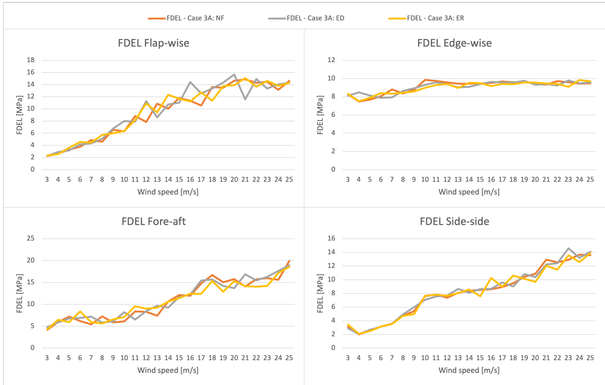
Figure 5.17: FDEL for wind speeds 3 to 25 m/s for all scenarios in case 3A. The grid frequency inputs are denoted as NF for the normal grid frequency, ED for the extreme deviation grid frequency and ER for the extreme RoCoF.
