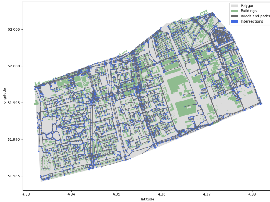
Figure 7.1: The street network returned from OpenStreetMap using OSMnx and the defined polygon
