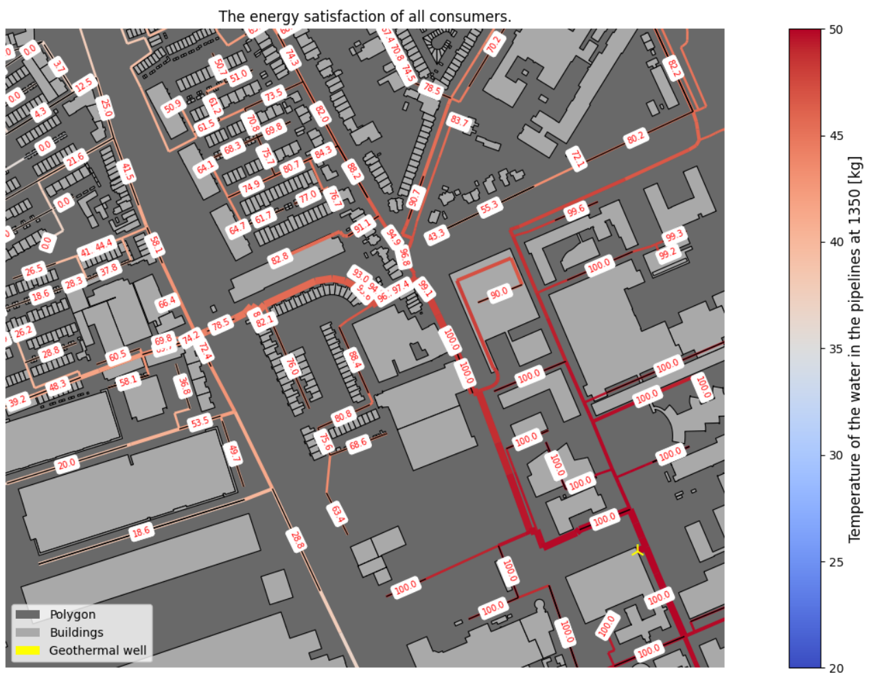
Figure 6.6: Demand satisfaction in a district heating network.
