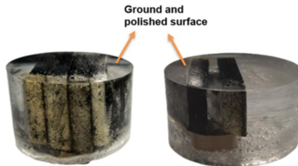
**Figure 4.9:** Ground and polished samples.
