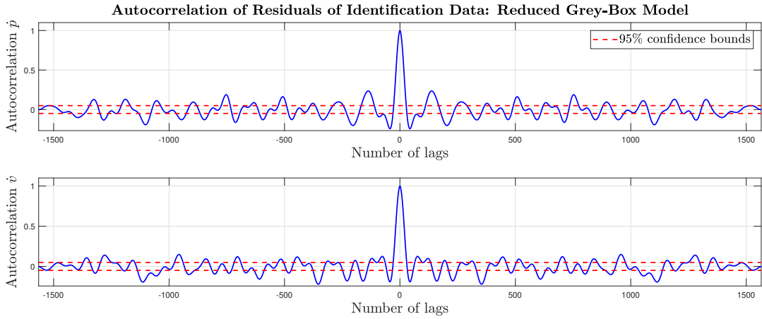
Figure 8.10: Autocorrelation plot of the residuals of the estimation shown in Figure 8.9. For the estimation two doublets of the maneuver shown in Figure 7.7 as the identification data and the reduced grey-box state-space system shown in Equation 8.4 as the model structure.
