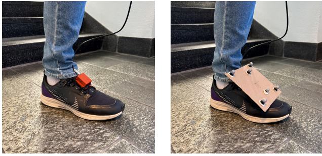
Figure 2. The experimental setup used to validate the proposed algorithm (left) and the visual markers fixed on top of the IMU for collecting the ground truth data (right).
