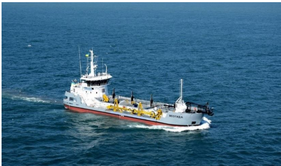
Figure 1: Trailing suction hopper dredger manufactured by Damen Shipyards
