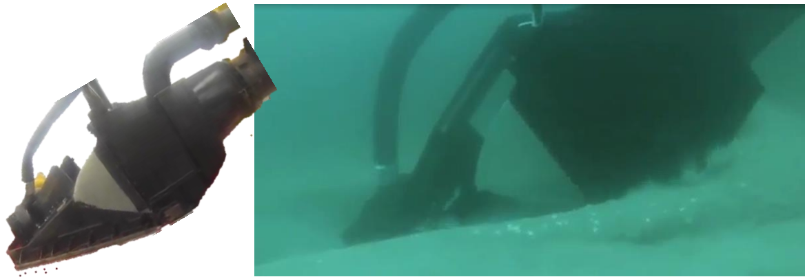
Figure 59: Image of a video recording of working draghead at 1.3 knots (0.67 m/s), lower suction pipe angle 45°
