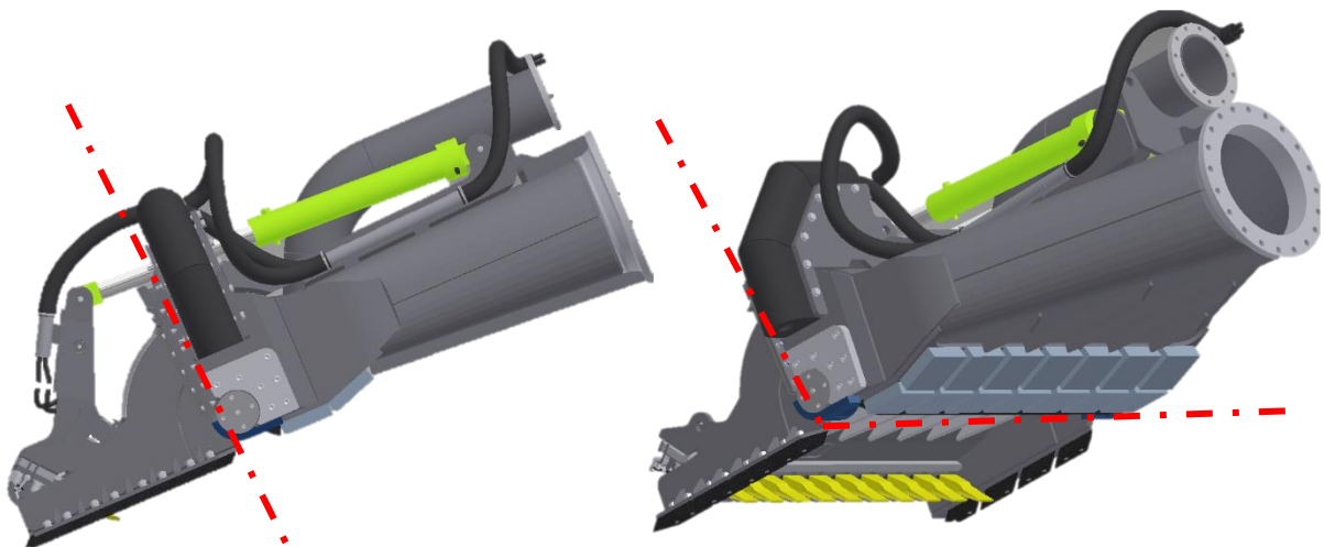
Figure 40: Sideview of a draghead configuration with a hydraulic cylinder
