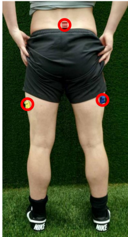
Figure 1.1: Sensor placement [10]: The sensors were placed at the sacrum and iliotibial tracts.
