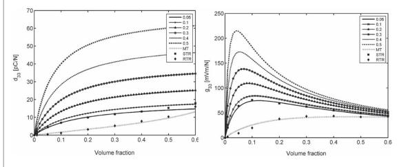
**Figure 2.** Test results for measured  $d_{33}$  and  $g_{33}$  for structured and random with the predicted values of the VPMT method, indicated with a value for  $c_{VP}$ , the MT method, structured composite test results (STR), and random composite test results (RTR). Material parameters are based on PZT-5A and fully cured polyurethane resin (Crystal Clear 202). Material properties as defined in the ComSol material database [40].
