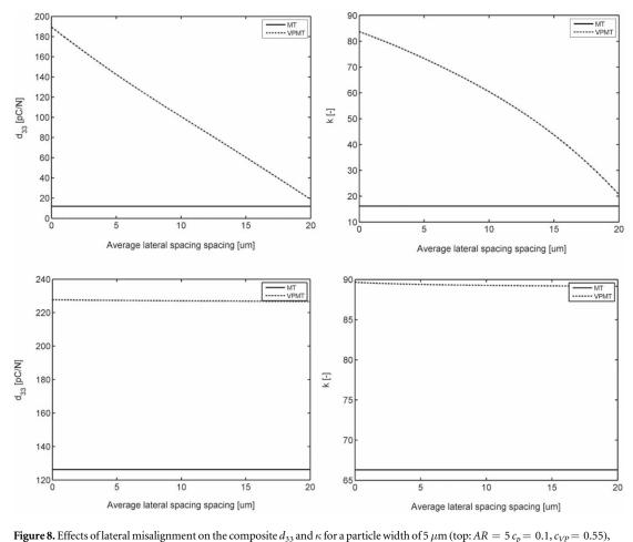
Figure 8. Effects of lateral misalignment on the composite  $a_{33}$  and  $\kappa$  for a particle width of 5  $\mu$ m (top:  $AR = 5 c_p = 0$ . (bottom:  $AR = 20 c_p = 0.1, c_{VP} = 0.55^* \eta_{lat}$ ).
