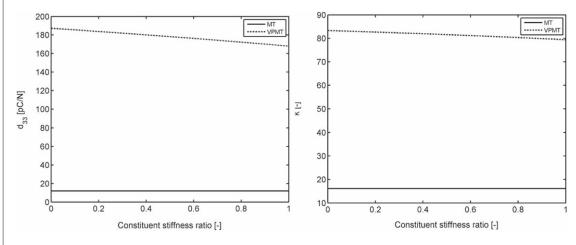
**Figure 12.** Effect of particle overlap on the composite  $d_{33}$  and  $\kappa$  as a function of  $Y_m/Y_p$  ratio (AR = 5,  $c_p = 0.1$ ,  $c_{VP} = 0.55 * \eta_{ob} l_{ol} = 0.3$ ,  $l_{olat} = 0.3$ ).
