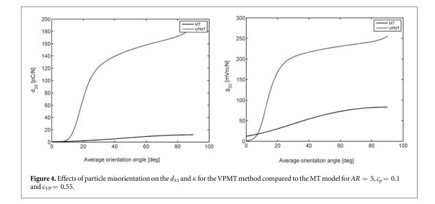
calculated results for the VPMT method are lower than those of the MT method for structured composites as long as the misorientation angle is less than 10<sup>0</sup> the conventional MT model describes the properties adequately. For higher misorientation angles the MT method rather over-estimates the properties.
