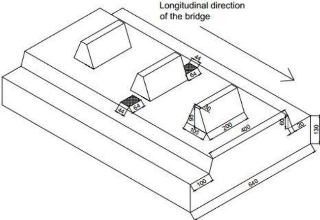
Figure 4-3 - Section of lower rail track showing two 44mmx64mm area
