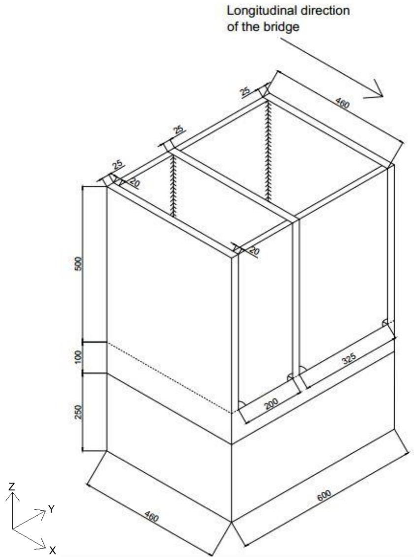
Figure 4-8 - New configuration of model, load located mid-section
