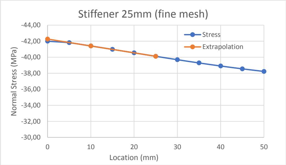
Figure 6-3 - Normal stresses on stiffener 2 and hot-spot extrapolation
