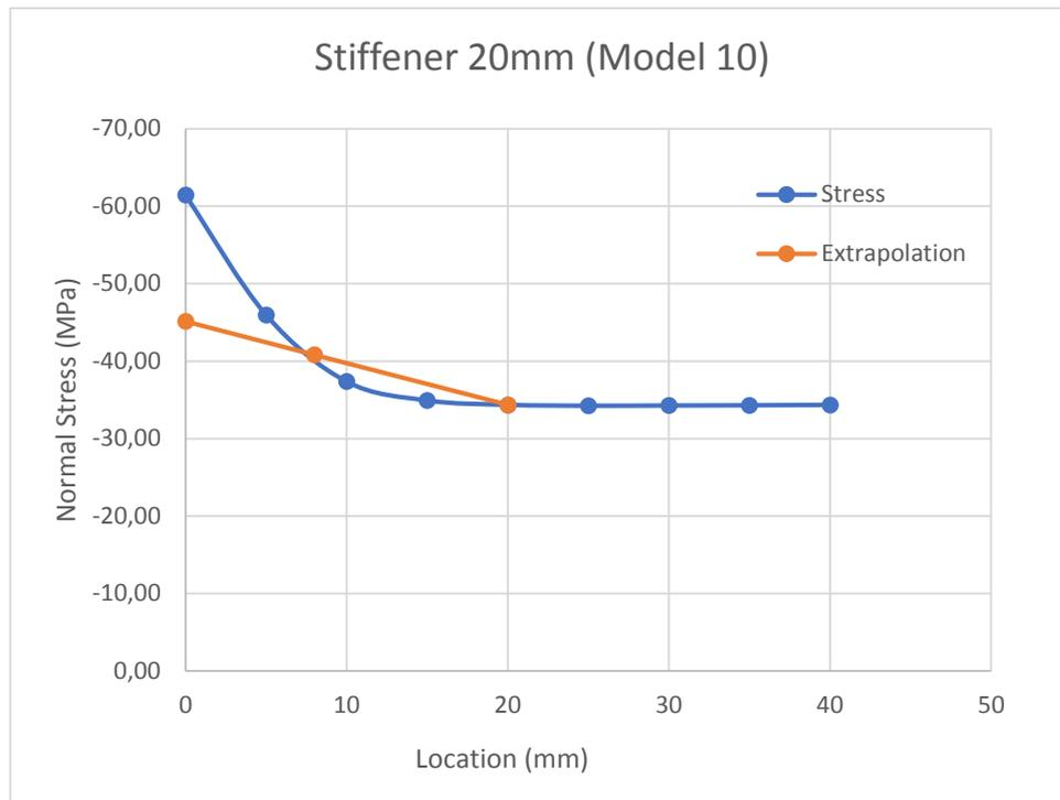
Figure 5-14 - Normal stresses on stiffener 1 and hot-spot extrapolation (Model 10)
