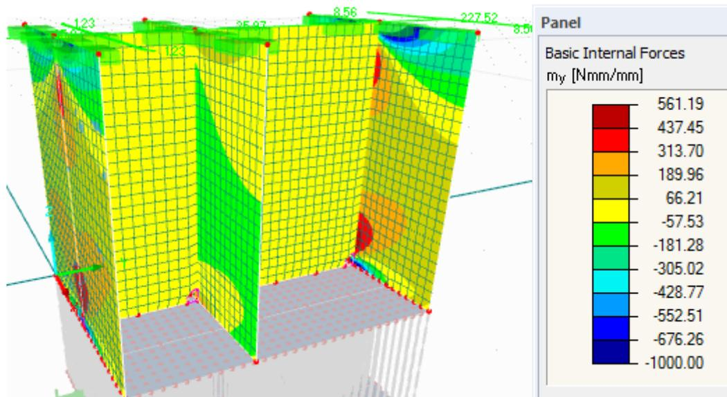
Figure 5-3 - Internal forces my (bending) on stiffeners
