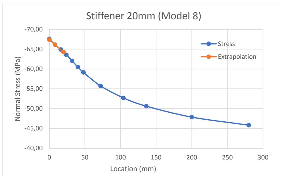
Figure 5-9 - Normal stresses on stiffener 1 and hot-spot extrapolation (Model 8)
