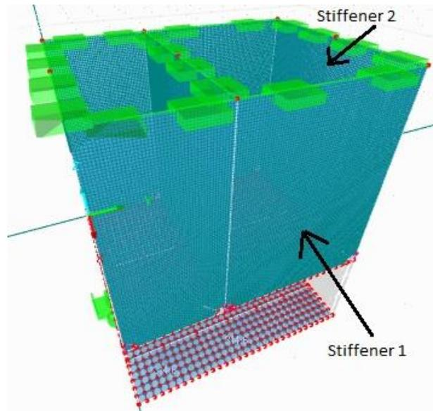
Figure 5-13 - Model with load between stiffeners (Model 10)
