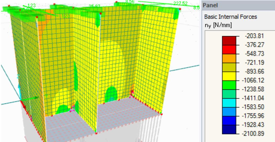
Figure 5-2 - Internal forces  $n_y$  (axial) on stiffeners
