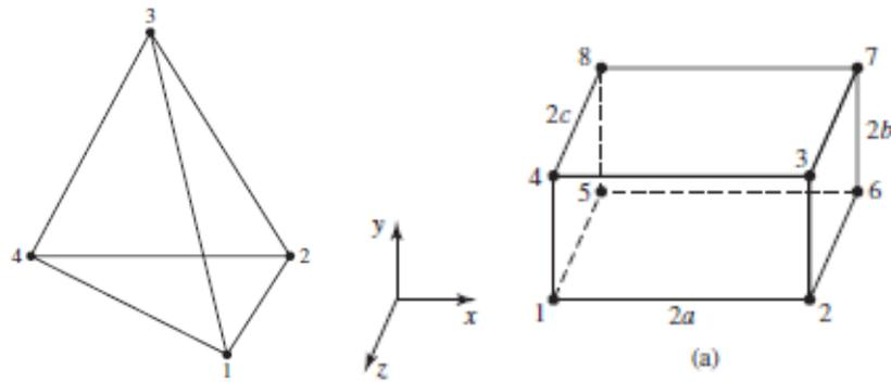
Figure 2-11 - Tetrahedral and Brick elements (4- and 8-noded) [17]
