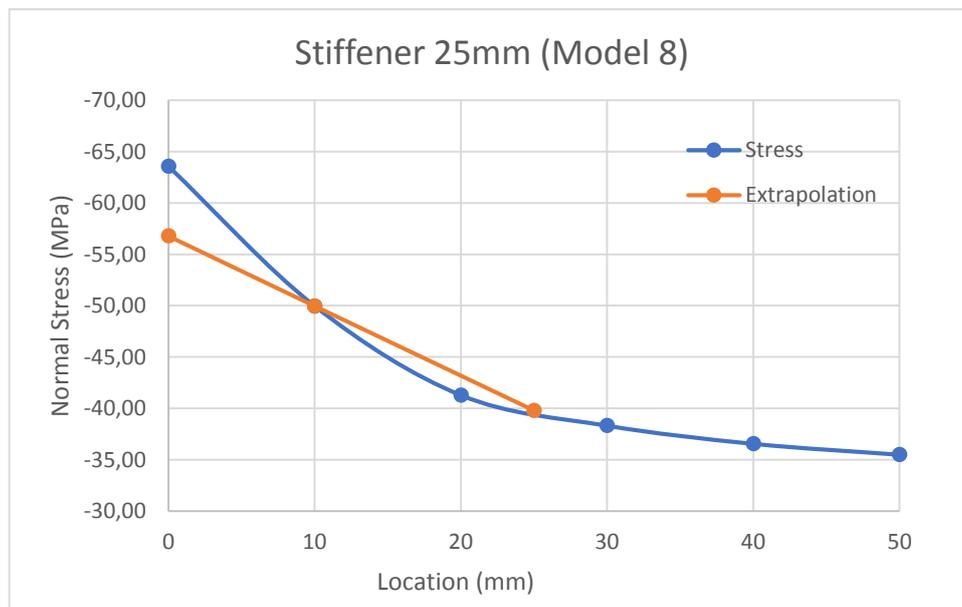
Figure 5-10 - Normal stresses on stiffener 2 and hot-spot extrapolation (Model 8)
