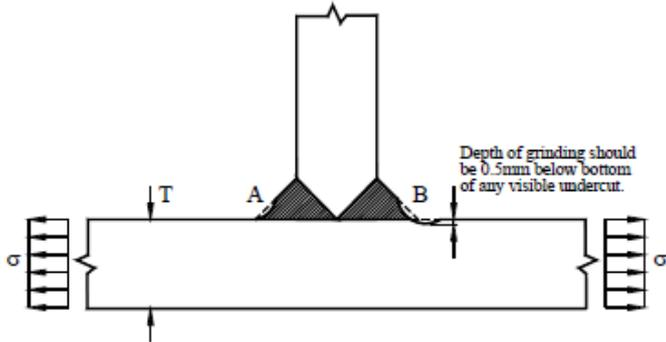
Figure 2-14 - Example of Weld Toe Grinding [6]
