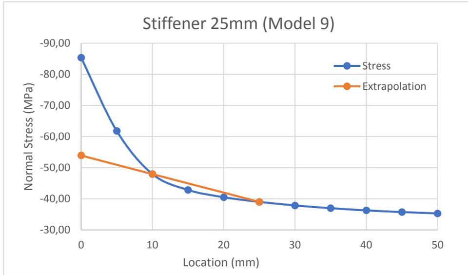
Figure 5-12 - Normal stresses on stiffener 2 and hot-spot extrapolation (Model 9)
