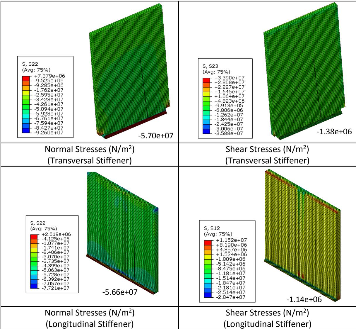
The following figures show the stresses on the transversal stiffener under a side surface boundary condition caused by the presence of the rail track itself.
