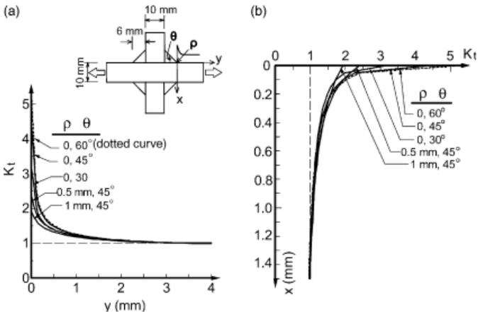
Figure 2-9 - Stresses distribution in weld toe region: (a) along surface; (b) through thickness [30]
