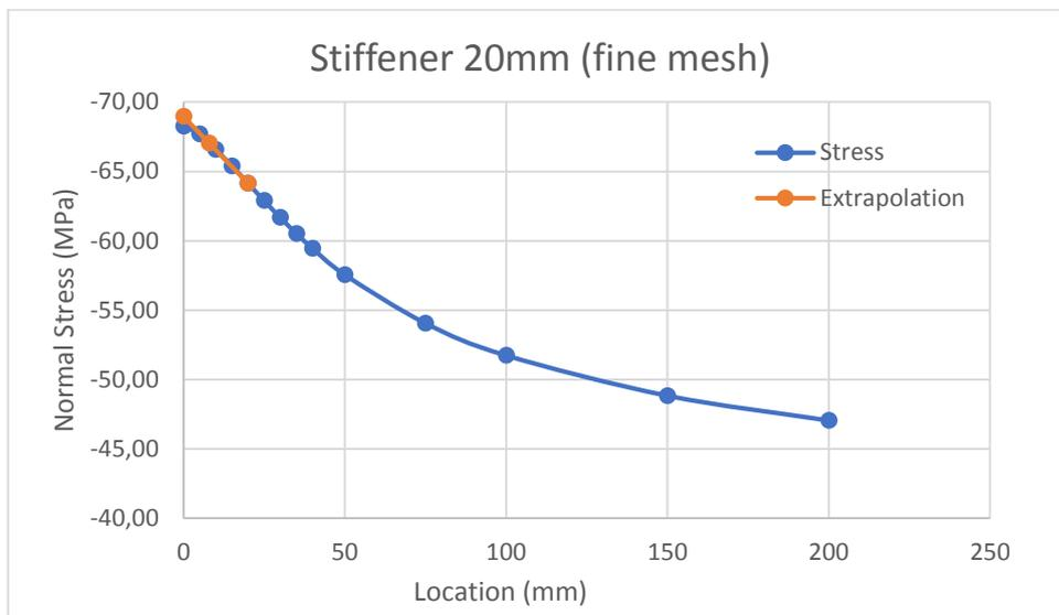
Figure 6-2 - Normal stresses on stiffener 1 and hot-spot extrapolation
