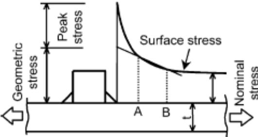
Figure 2-5 - Example of stress curve obtained through modelling [30]
