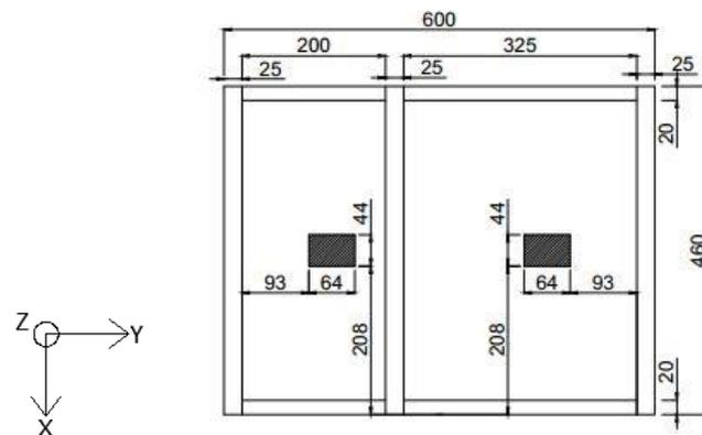
Figure 4-9 - Top view of the detail (shadow represents the locations of the forces)
