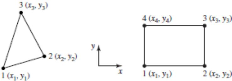
Figure 2-10 - Triangular and rectangular elements (3- and 4-noded) [17]
