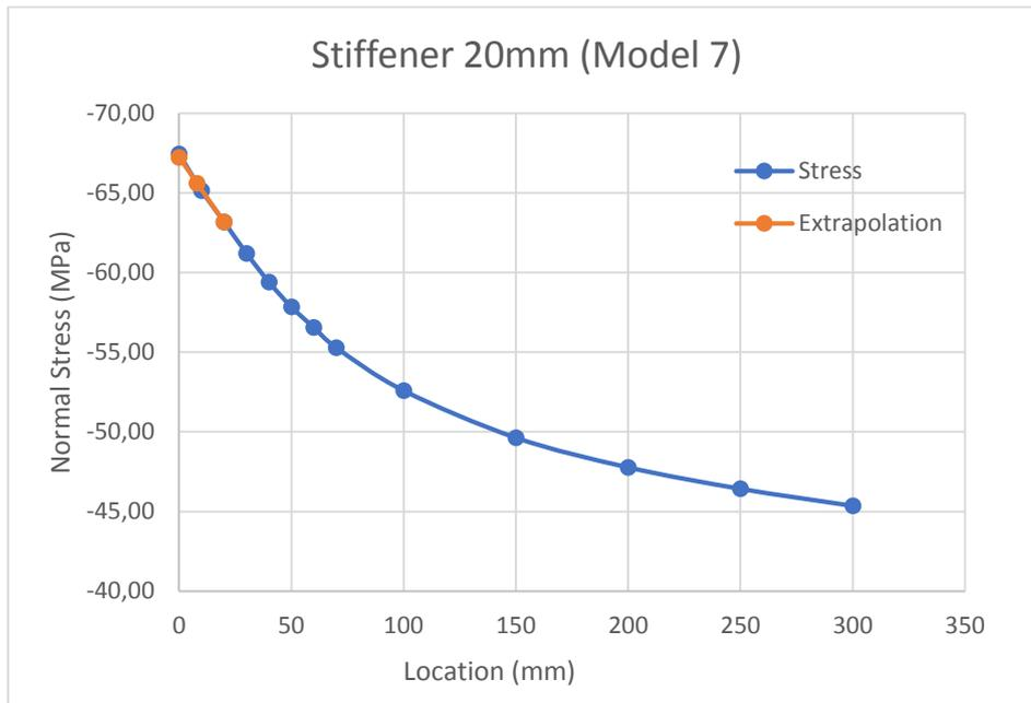
Figure 5-7 - Normal stresses on stiffener 1 and hot-spot extrapolation (Model 7)
