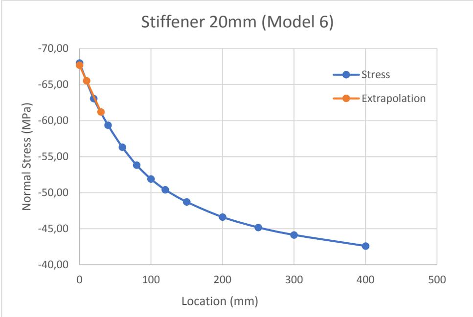
Figure 5-5 - Normal stresses on stiffener 1 and hot-spot extrapolation (Model 6)
