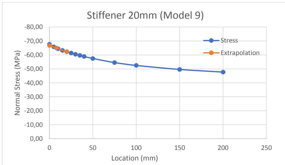
Figure 5-11 - Normal stresses on stiffener 1 and hot-spot extrapolation (Model 9)
