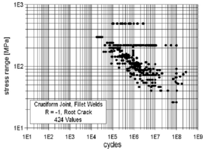
Figure 2-1 - Typical data obtained for a S-N curve [15]
