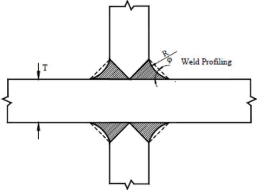
Figure 2-15 - Example of Weld Profiling [6]
