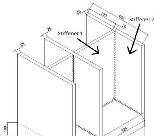
Figure 5-4 - Critical stiffener 1 (transversal) and 2 (longitudinal)
