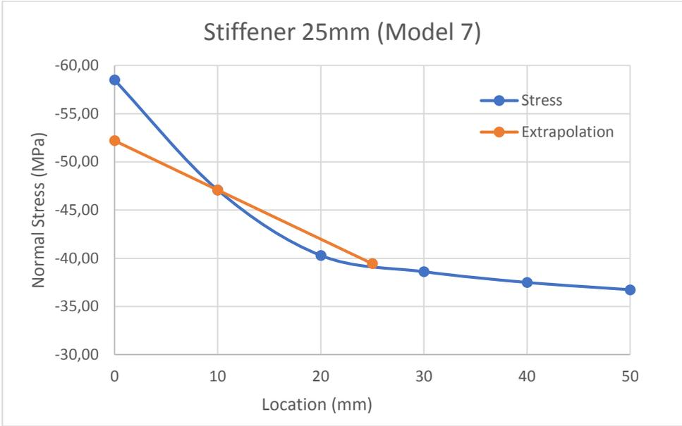
Figure 5-8 - Normal stresses on stiffener 2 and hot-spot extrapolation (Model 7)
