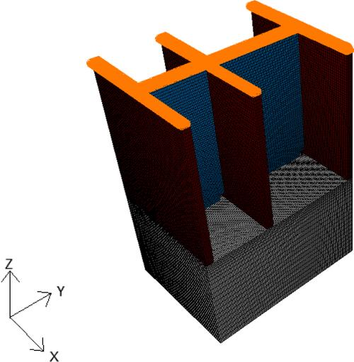
Figure 6-7 - Model with solid elements (Fine mesh)
