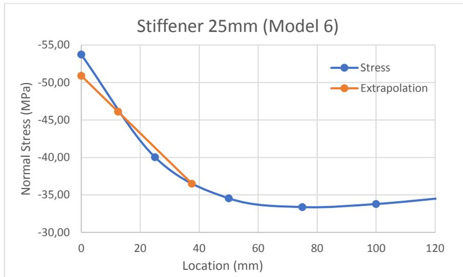
Figure 5-6 - Normal stresses on stiffener 2 and hot-spot extrapolation (Model 6)
