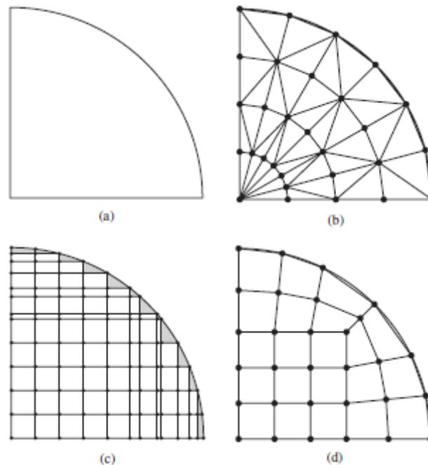
Figure 2-12 - Meshing of a surface [17]
