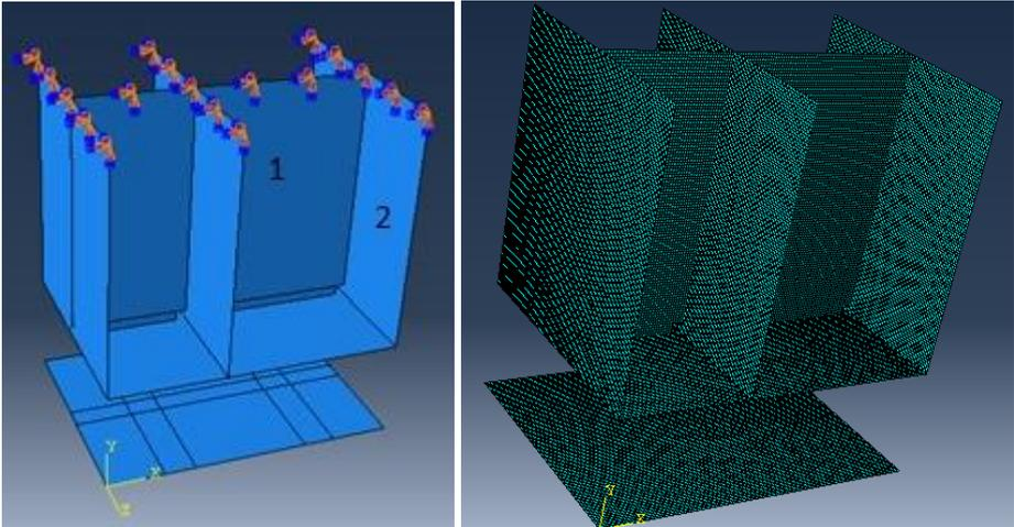
Figure 6-1 - Model with shell elements and meshed configuration
