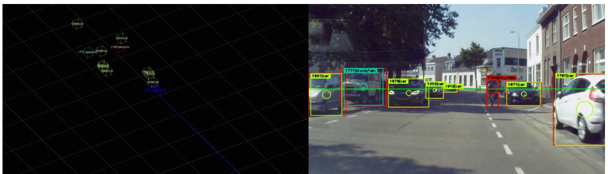
Figure A.6 Detection and tracking of various road users using cameras (right), resulting in a 3-dimensional world view (left) that allows assessment of traffic density and complexity, relative distances and speeds, and derived measures.
