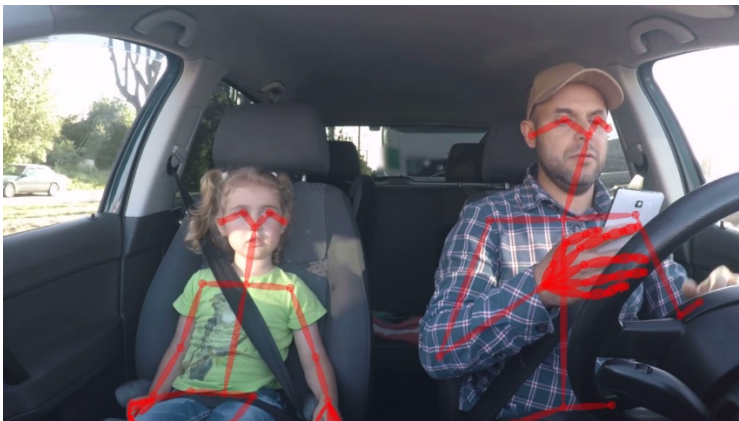
Figure A.4 Body pose information extracted from an inward-looking camera, allowing extraction of information on what the driver is doing with his hands.
