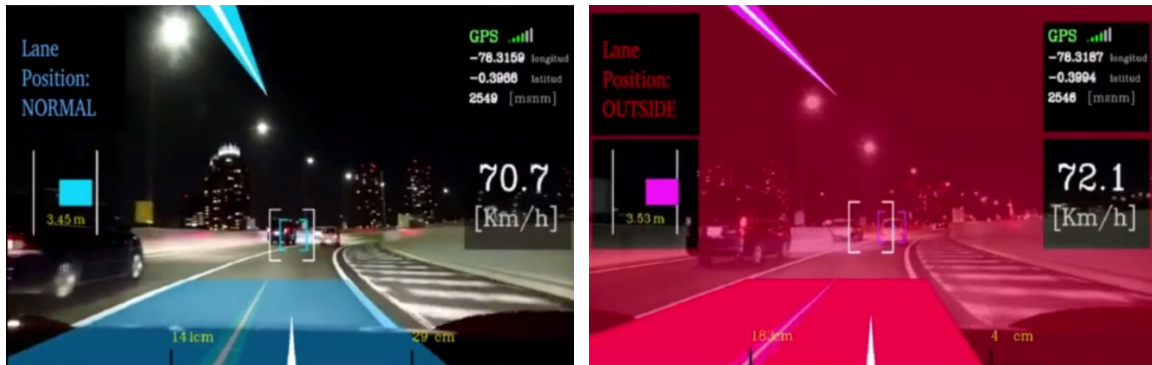
Figure A.7 Illustration of lane position and lane departure information. Left: lane position within the acceptable limits; right: lane position outside the acceptable limits, i.e. a lane departure instance.
