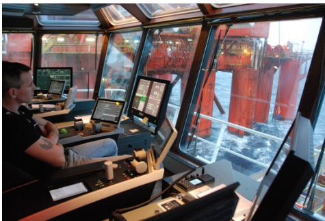
Figure 5.10 DP operator monitoring the DP system on a supply vessel delivering cargo to a drilling rig. The DP system controls, heading, sway and surge. (Photo: Stig Olav Skeie/Kongsberg Maritime).
