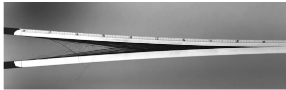
Fig. 4. Fibre bridging in delamination growth of carbon fibre reinforced composites.
