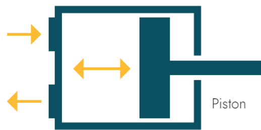
Figure 2-6: Working principle of a reciprocating compressor. Through reciprocating motion of the piston the gas is compressed [22].
