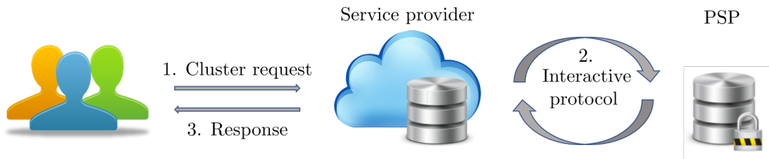
Figure 4.1: Users can request a clustering result to a service provider, which only receives encrypted data. A privacy service provider (PSP) who owns the decryption key is required to facilitate the computations.
