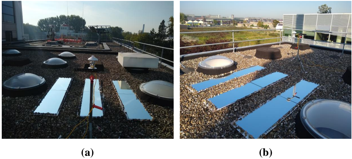
Figure 5.7: The used experimental setup for measuring specular reflections on the PVMD monitoring roof.
