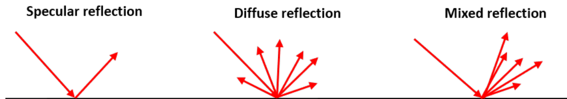
Figure 2.7: Specular, diffuse and mixed reflection shown in a schematic manner[9].
