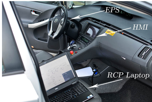
Figure 5-1: Interior of the vehicle.
