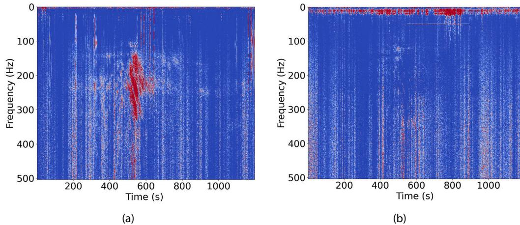
**Fig. 3.** a): Frequency content of water, calculated by subtracting channel 450, buried in mud and channel 610, located in water, and b) frequency content of mud, calculated by subtracting channel 610 from channel 450.
