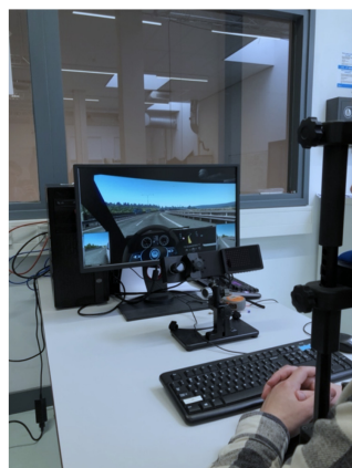
Figure 1. Experimental setup. Shown from back to front is the monitor for displaying the videos, the eye-tracker camera with infrared illuminator, the keyboard used for pressing the spacebar and arrow keys, and the head support.
