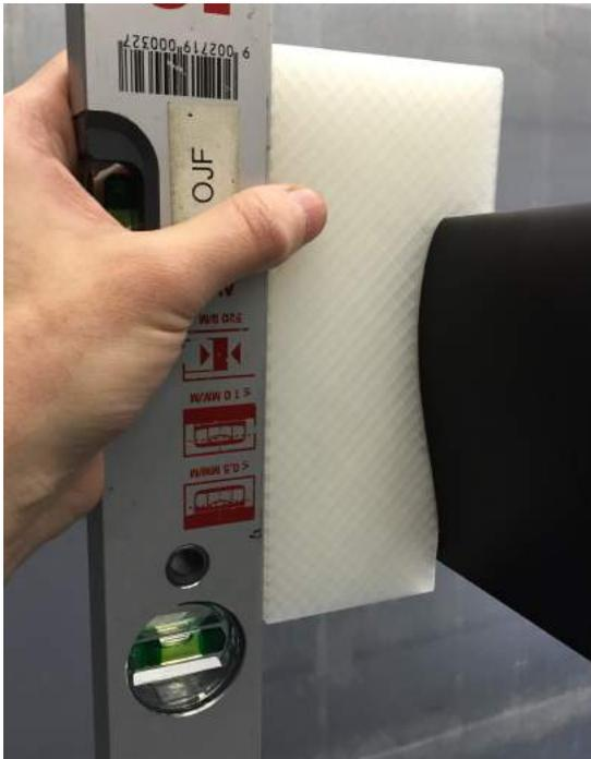
(a) Bubble level being used with the 3D mould
