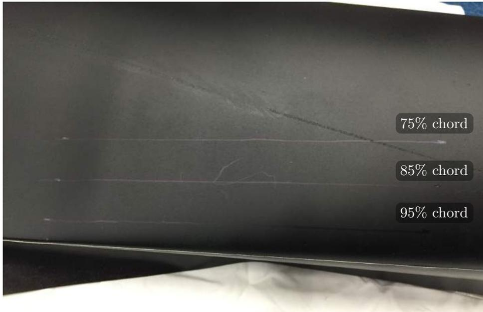
**Figure 4.7:** The three different flap locations marked with pencil on the blade
