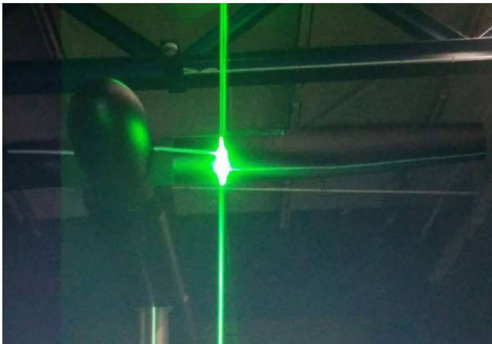
**Figure 7.4:** This picture clearly shows the extent of light being reflected from the wind turbine model blade. The reflected region is not usable for the analysis.
