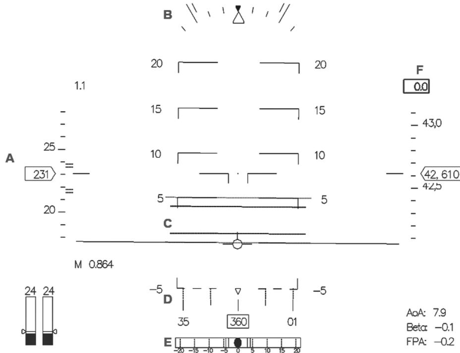
**Fig. 4 Primary flight display HUD view, with at A: Velocity indicator with (stippled) target margins; B: Roll angle indicator with target margins; C: Flight Path Marker with (stippled) target margins; D: Sideslip angle indicator with target margins; E: Heading indicator with (stippled) target margins; F: maneuver timer.**
