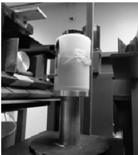
Fig. 5. The large food sample being counted after neutron activation
