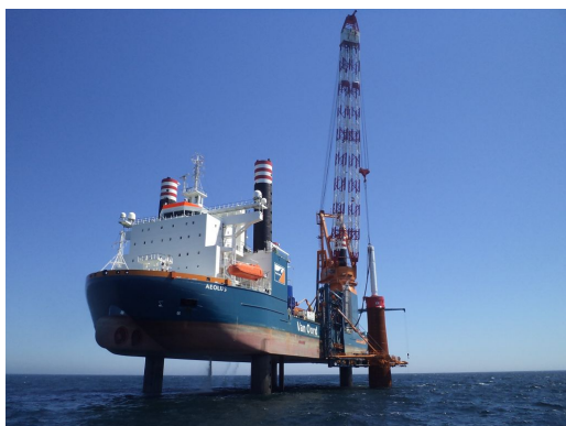
Figure 7: Offshore installation vessel Aeolus.
