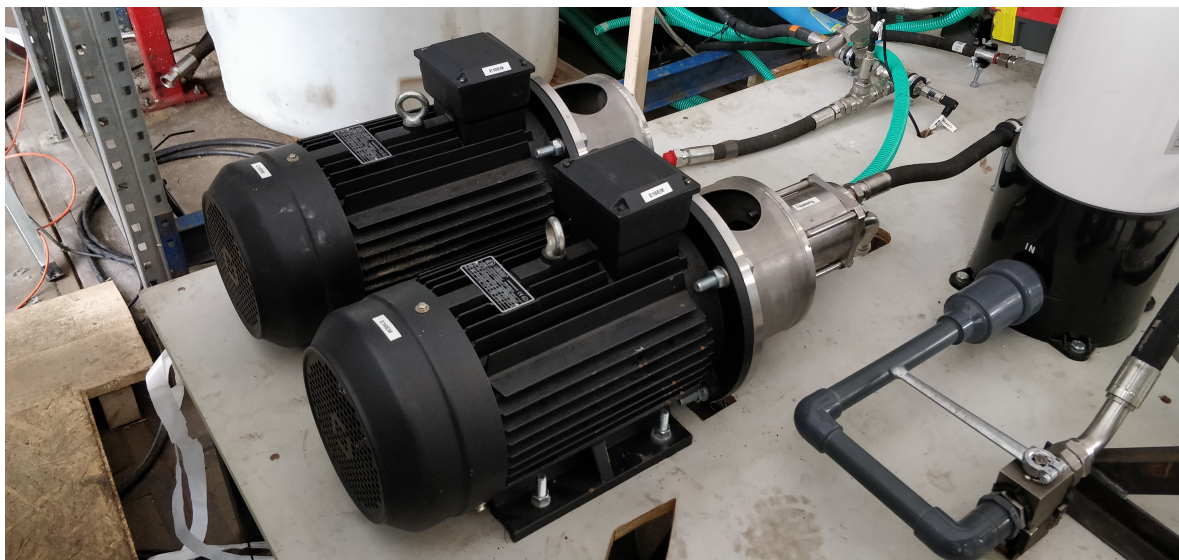
Figure 7-3: The wind turbines are represented by an electric motor and hydraulic pump, connected by a ROTEX flexible jaw coupling in an aluminium lantern housing.
