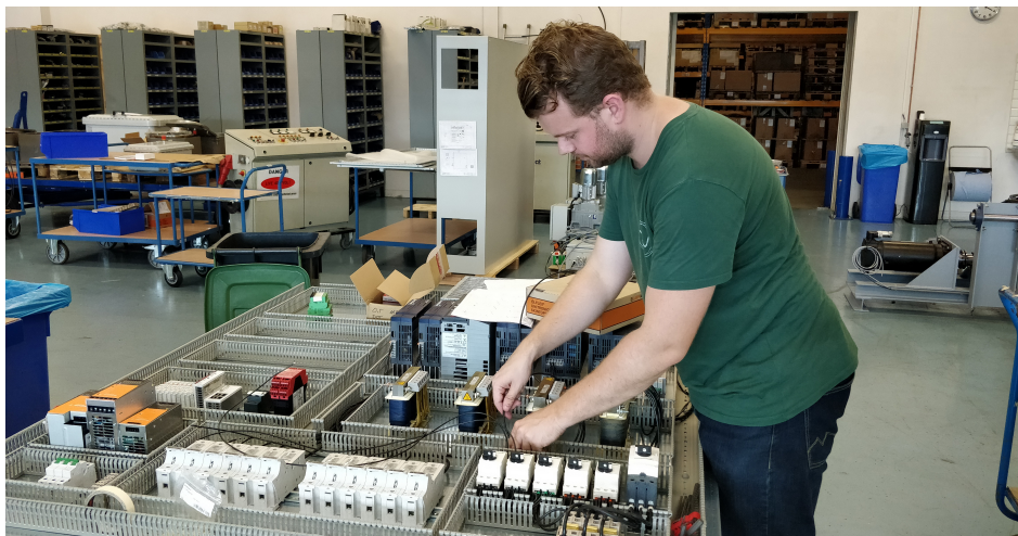
Figure F-1: The manufacturing process of the electrical cabinet at Elsto Drives & Controls.
