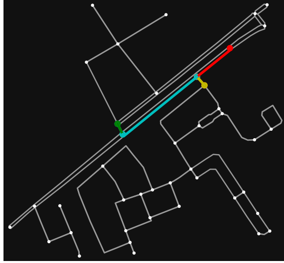
Figure 6.1. Map of toy problem’s pedestrian G_{\text{start}} including the decision variable edges (colored edges). The number of colored edges is less than a as some of them are of the same two-way street but represent different directions.
