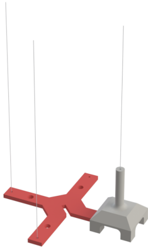
Figure 11: 3D printed holders (grey) are used during the manufacturing process to assure a straight and perpendicular glue connection between the steel cross and the wire flexure during glue curing.
