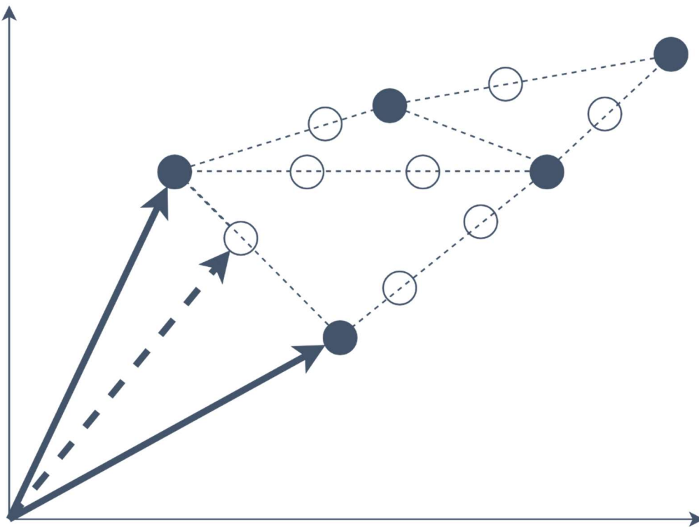
Figure 17: SMOTE: the five solidly filled points are the 'real' data. In between all data points, new 'synthetic' points are created on a random distance between the two 'real' points (Khurkhuriya, 2018)
