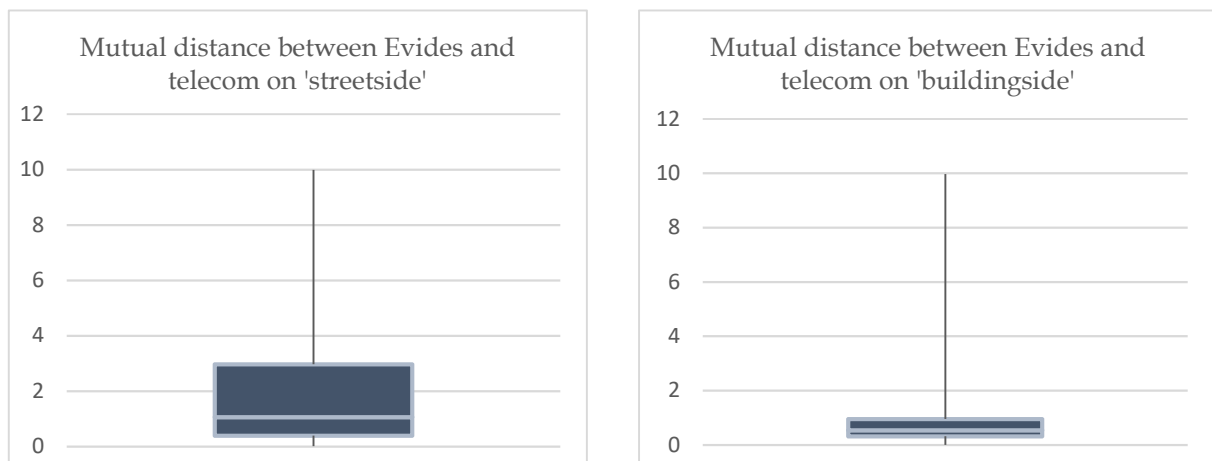
Figure 24: The distance from the telecom cable to the Evides main for the two 'sides' are compared. It was found that the telecom cables are +/- 50 cm closer to the Evides main on the building sides than on the street sides.
