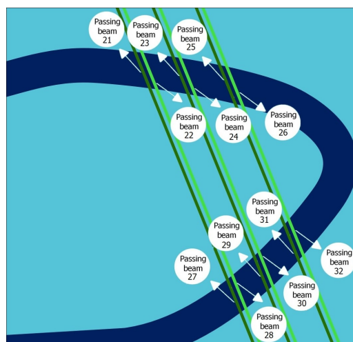
Figure 4.6: The river could have been passed by the satellite more than once due to the shape of the river. For each location ICESat-2 passes the river, a unique ID should be assigned.
