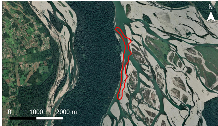
Figure 6.2: The red line shows the boundary of an object in the lake mask. Some lakes in the lake mask turn out to be parts of a river, water surface heights for rivers should be determined with a different method.
