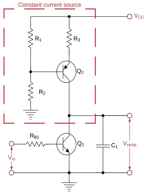
Figure 7.2: The schematic of the ramp generator.
