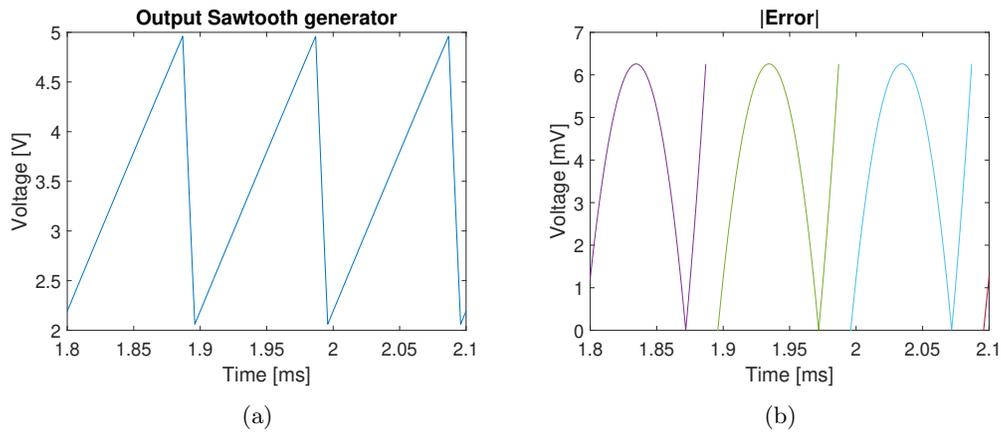
Figure 9.2: (a) The output waveform of the sawtooth generator with selected components and (b) the absolute error of the output compared to a linear approximation.
