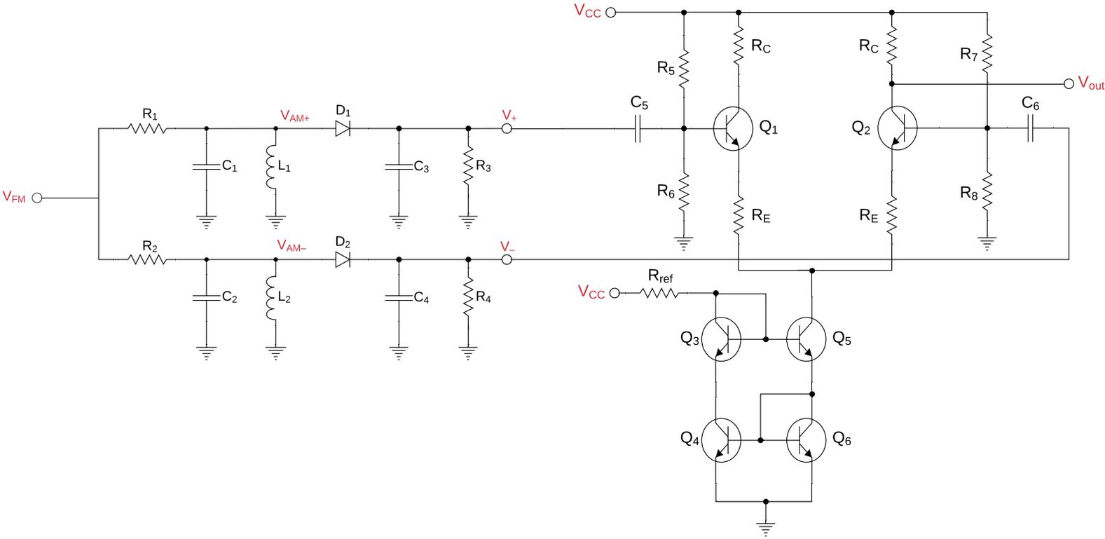
Figure B.2: The schematic of the FM detector.
