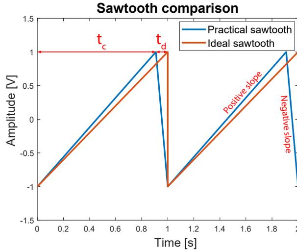
Figure 5.1: The difference between a mathematical sawtooth and a realistic sawtooth.
