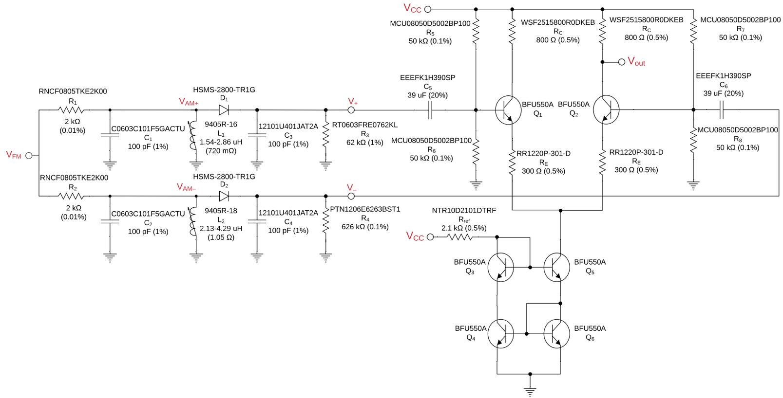
Figure H.2: The schematic of the FM detector with the chosen components.
