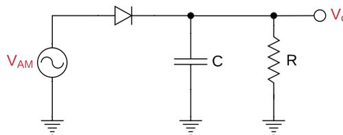
Figure 13.7: The envelope detector.
