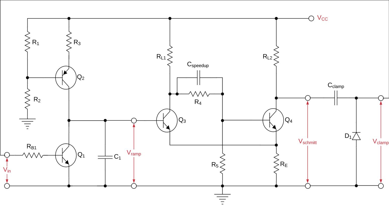
Figure B.1: The schematic of the sawtooth generator.
