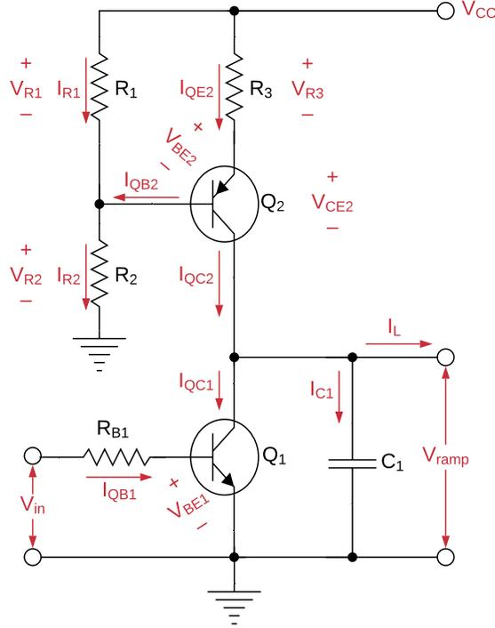
Figure 8.1: The schematic of the constant current ramp generator.
