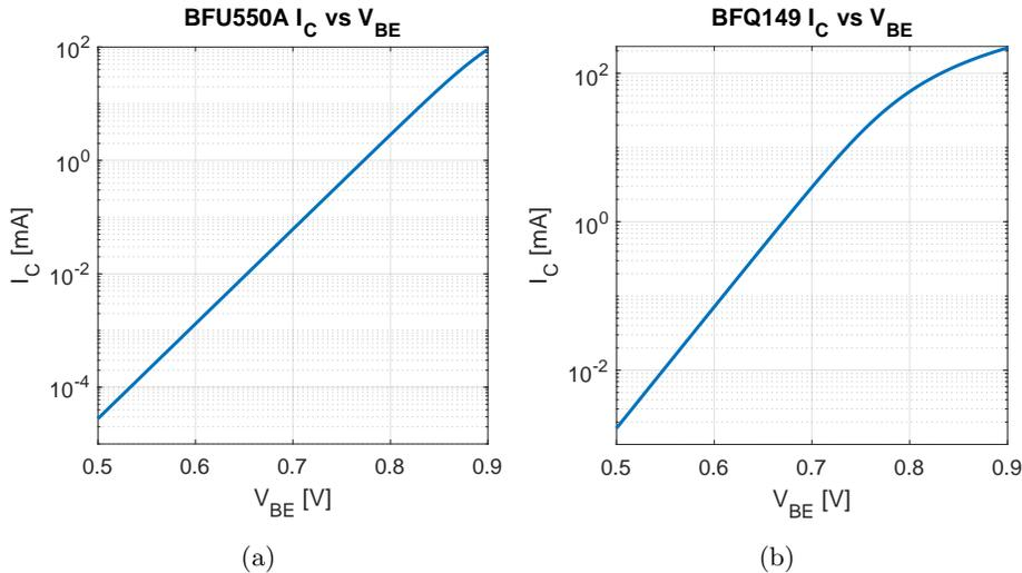
Figure 4.1: The  $I_C$  vs  $V_{BE}$  curve of the: (a) BFU550A and (b) BFQ149 for  $V_{CE} = 8$  V.
