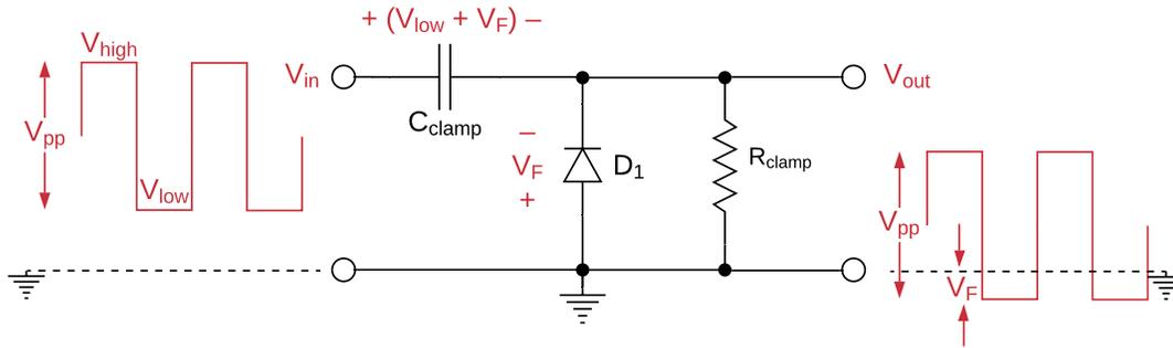
Figure 7.5: The schematic of a clamping circuit together with its input/output characteristic.
