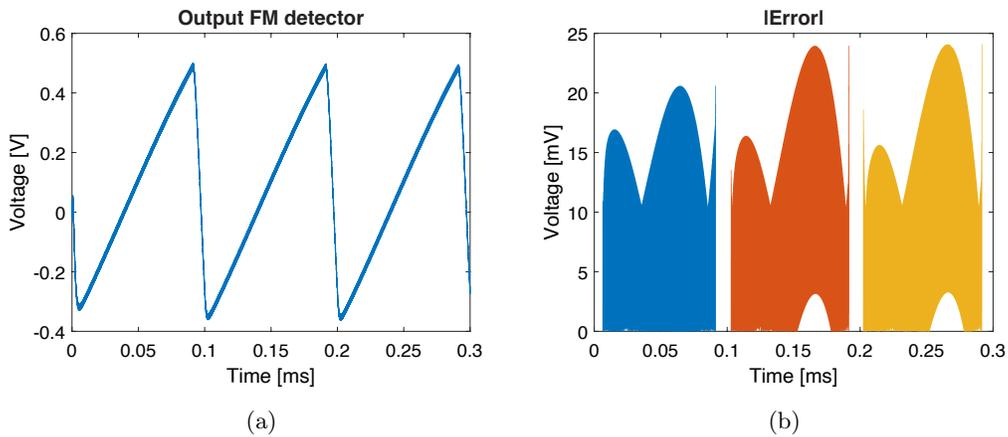
Figure E.3: (a) The output of the baseband amplifier together with the FM detector (b) the absolute error of the output compared to a linear approximation.
