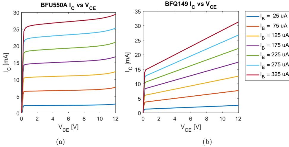
Figure F.1: The  $I_C$  vs  $V_{CE}$  curve of the: (a) BFU550A and (b) BFQ149.
