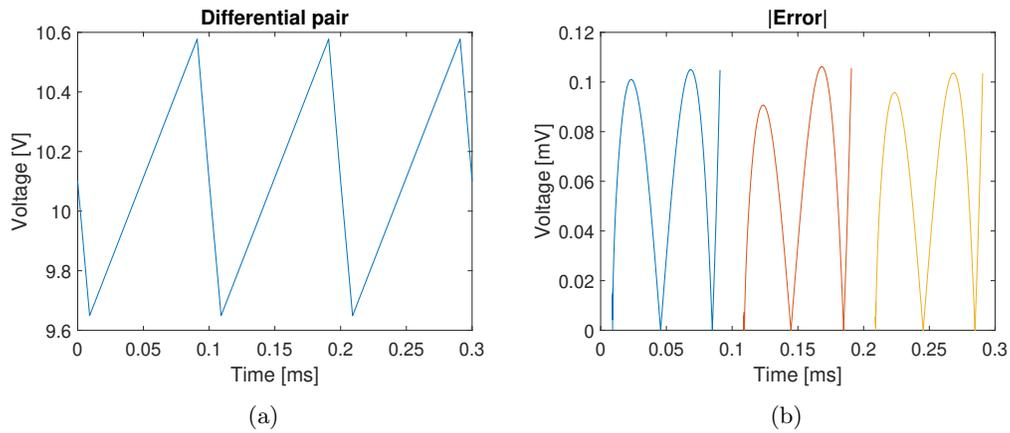
Figure 15.2: (a) The output of the differential-to-single-ended converter and (b) the absolute error of the output compared to a linear approximation.
