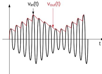
Figure 13.8: The working principle of an envelope detector.
