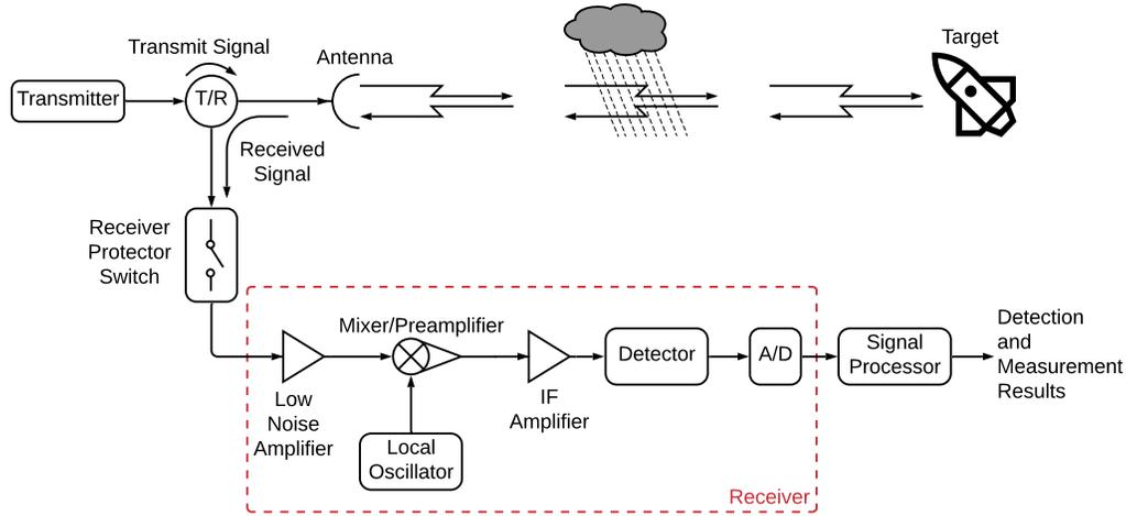
Figure 1.1: Major elements of the radar transmission/reception concept (based on [4]).
