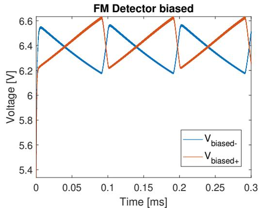
Figure D.4: The DC biased inputs of the differential-to-single-ended converter.
