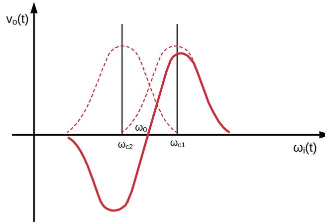
Figure 13.6: The magnitude response of a balanced detector.
