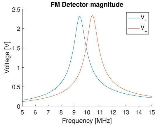
Figure D.1: The frequency response of the bandpass filters.
