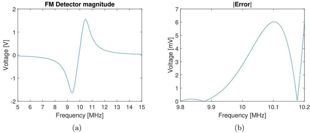
Figure 15.1: (a) The frequency response of the FM detector and (b) the absolute error of the frequency response compared to a linear approximation for the region of interest.
