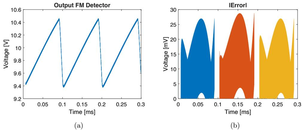
Figure 15.3: (a) The output waveform of the FM detector with calculated component values and (b) the absolute error of the output compared to a linear approximation.
