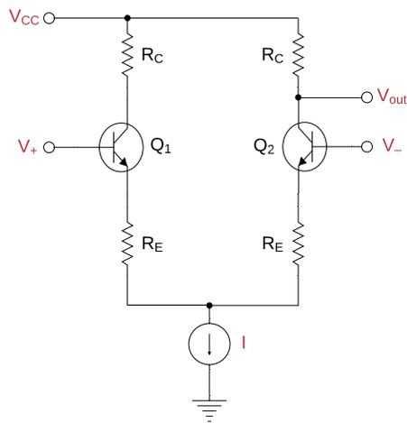
Figure 13.9: The schematic of a differential pair with emitter degeneration.
