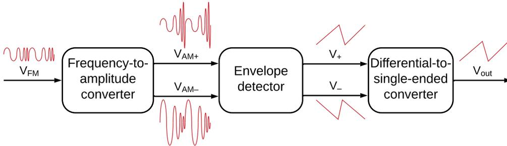
Figure 13.1: The block diagram of an FM detector.
