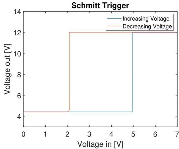
Figure C.1: The input/output relationship of the Schmitt trigger.
