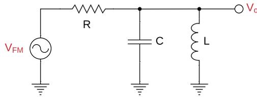
Figure 13.2: A simple RLC circuit implemented as a bandpass filter.
