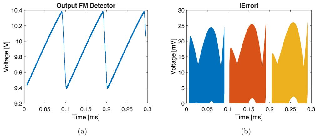
Figure 15.4: (a) The output waveform of the FM detector with selected components and (b) the absolute error of the output compared to a linear approximation.
