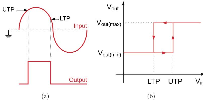
Figure 7.3: (a) The output waveform of a Schmitt trigger for a sinusoidal input and (b) The hysteresis of the Schmitt trigger, where the input/output relationship is dependent on the path.
