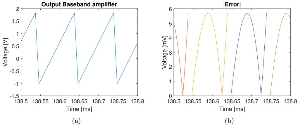
Figure E.1: (a) The output of the baseband amplifier together with the sawtooth generator (b) the absolute error of the output compared to a linear approximation.
