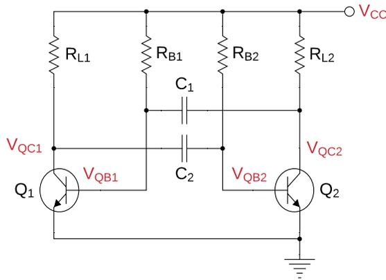
Figure 6.1: A schematic of an astable multivibrator.
