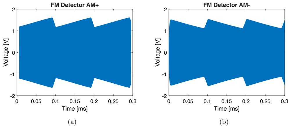
Figure D.2: (a) The output of the first bandpass filter, which is responsible for the positive input
