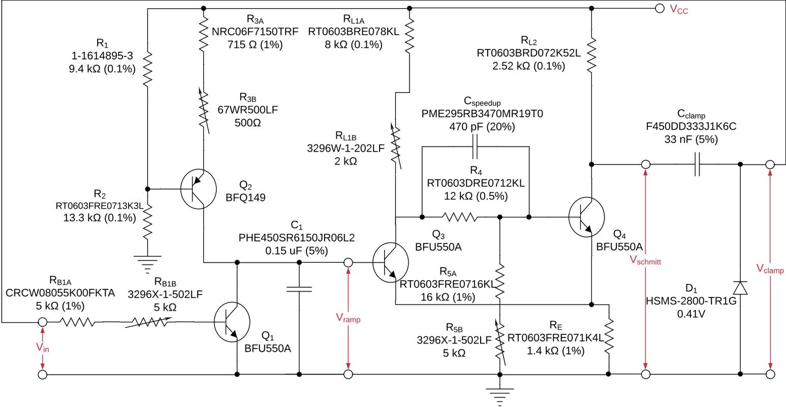
Figure H.1: The schematic of the sawtooth generator with the chosen components.
