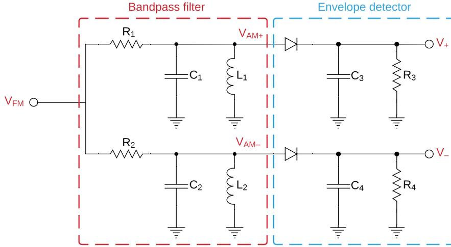
Figure 14.1: The schematic of a balanced slope detector.
