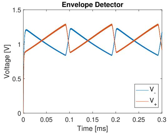
Figure D.3: The output of the envelope detectors.
