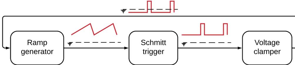
Figure 7.1: An overview of the sawtooth generator.
