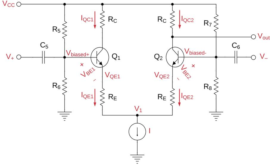
Figure 14.2: The schematic of the differential-to-single-ended converter.
