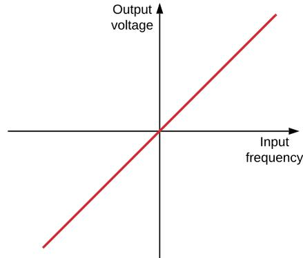
Figure 12.1: The characteristics of an FM detector.
