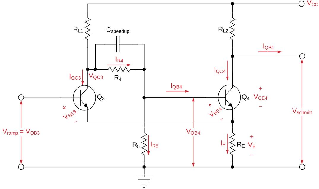
Figure 8.2: The schematic of the Schmitt trigger.
