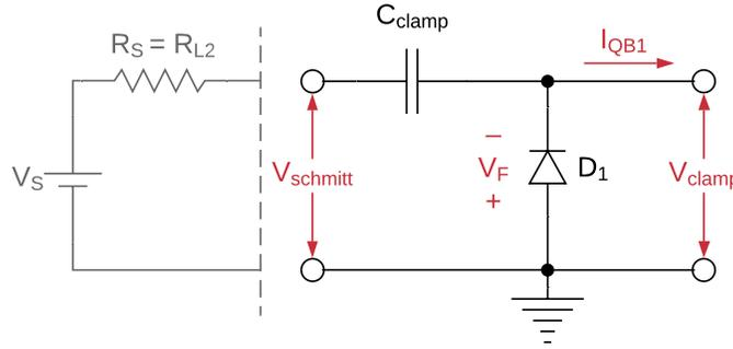
Figure 8.3: The schematic of the clamping circuit.
