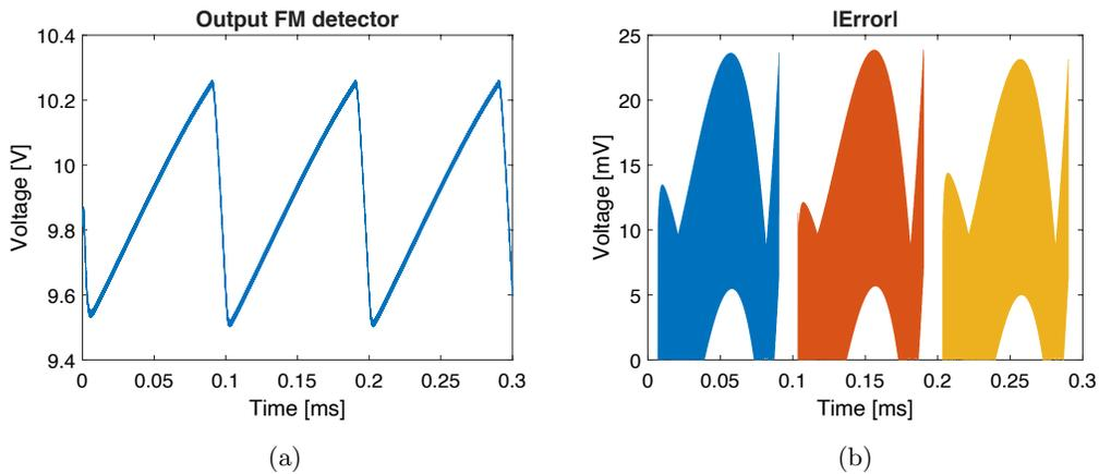
Figure E.2: (a) The output of the FM detector together with the IF amplifier (b) the absolute error of the output compared to a linear approximation.
