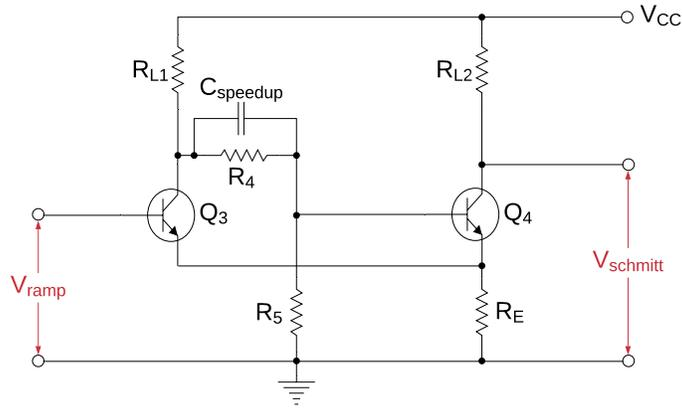
Figure 7.4: The BJT implementation of the Schmitt trigger.
