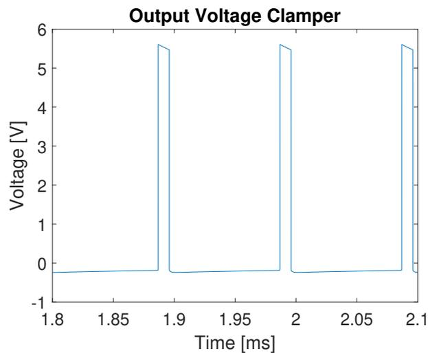
Figure C.3: The output of the voltage clamper.
