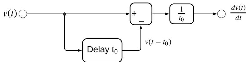
Figure 13.4: A block diagram implementation of a derivative.
