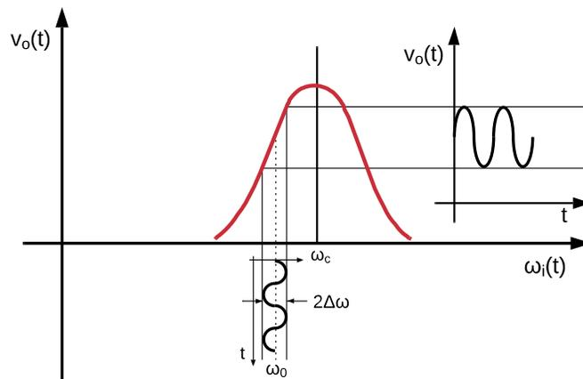
Figure 13.3: The working principle of a slope detector.
