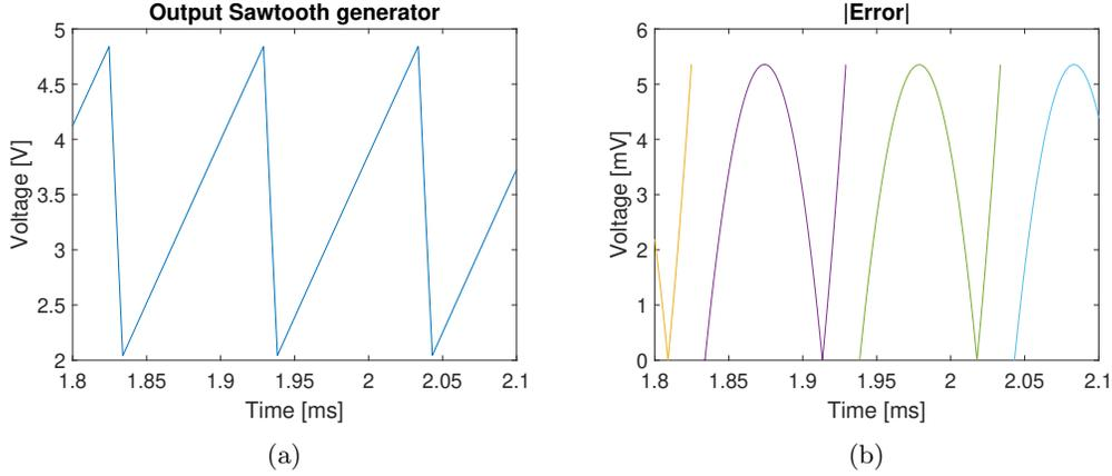
Figure 9.1: (a) The output waveform of the sawtooth generator with calculated values and (b) the absolute error of the output compared to a linear approximation.
