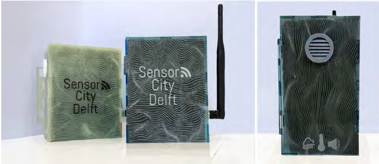
Figure 35: Final casing in 2 colors (left image). Ventilation piece and icons of measurements on the right side of the sensor box (right image)
