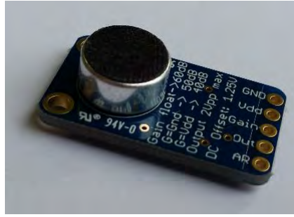
Figure 18: MAX9814 sound sensor
