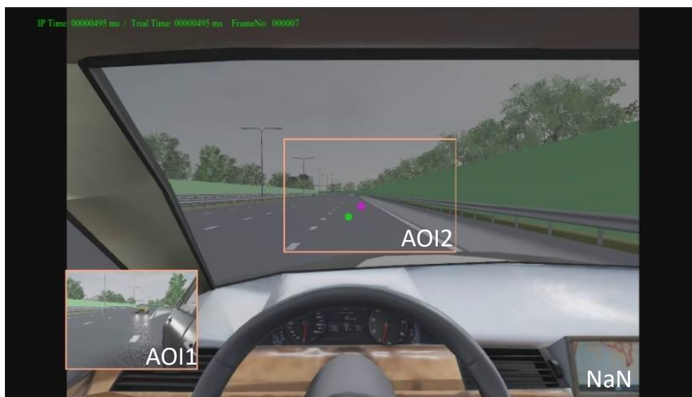
Figure 5: A snapshot of one trial for one participant in SR Research Dataviewer. The orange rectangles represent the two areas of interest (AOI) that were predefined for each condition, one being the side mirror (AOI1) and the second being the on-ramp (AOI2). If the participant did not look towards one of the areas of interests, "NaN" was outputted for that time frame. The purple and green dots are the gaze locations of the participant – green being the left eye and purple being the right eye. The rectangles, text and dots were not visible for the participant during the experiment.
