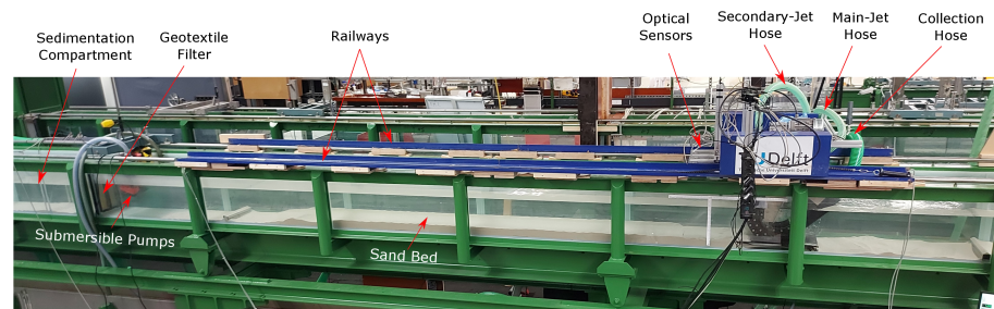
Figure 3. Front view of the experimental setup illustrating the equipment used in the experiments.
